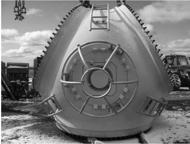
Figure 6.28 Typical rigid wind turbine hub. Photo by Paul Anderson. Reproduced under Creative Commons License
