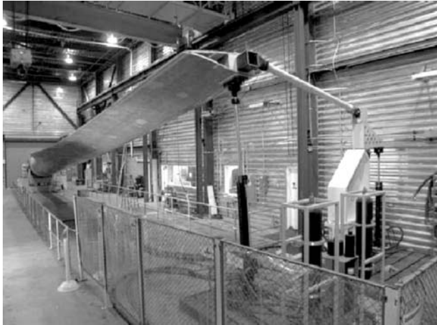
Figure 7.13 NREL's dual-axis forced displacement test set-up (White, 2004)
