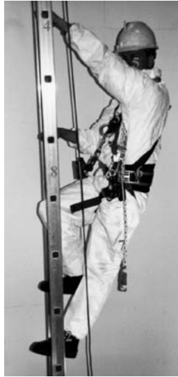
Figure 6.43 Tower climbing safety equipment. Reproduced by permission of Vestas Wind Systems A/S
