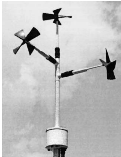
Figure 2.40 Propeller-type anemometer for measuring three wind velocity components
