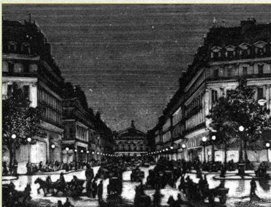
Yablochkov's AC arc-lighting system illuminating the Paris Exhibition of 1878
