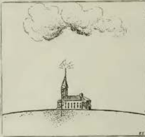
Fig. 4. Tesla Explains the Fallacy of the Franklin Pointed Lightning Rod, Here Illustrated, and Shows that Usually Such a Rod Could Not Draw Off the Electricity in a Single Cloud in Many Years. The Density of the Dots Indicates the Intensity of the Charges.
