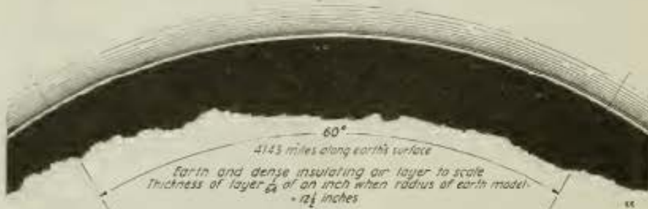
A Section of the Earth and Its Atmospheric Envelope Drawn to Scale. It is Obvious That the Hertzian Rays Cannot Traverse So Thin a Crack Between Two Conducting Surfaces For Any Considerable Distance, Without Being Absorbed, Says Dr. Tesla, in Discussing the Ether Space Wave Theory.
