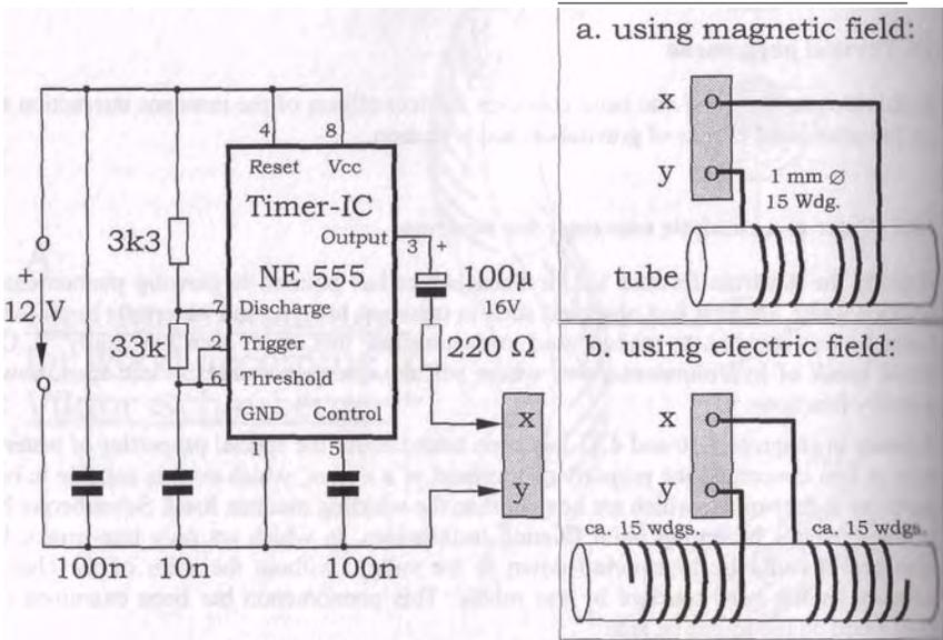
Fig. 18.1 C: Wiring diagram for a simple water processor with pulsed field (2 kHz rectangular signal)
