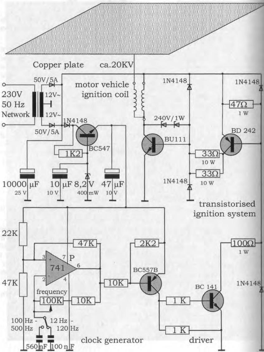
Fig. 19.4: Wiring diagram concerning the Kirlian device.
