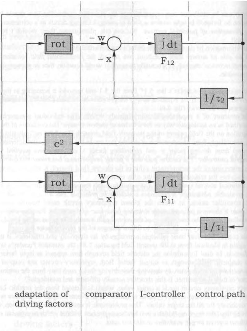
Fig. 8.7: Signal flow diagram of the fundamental field equation with adaptive structure.
