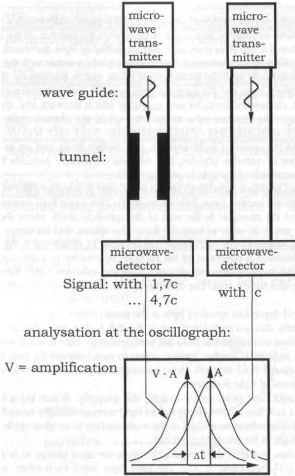
Fig. 6.14: The microwave experiment at the II. Physical Institute of the University of Cologne to measure speeds faster than light.<sup><i></sup>
