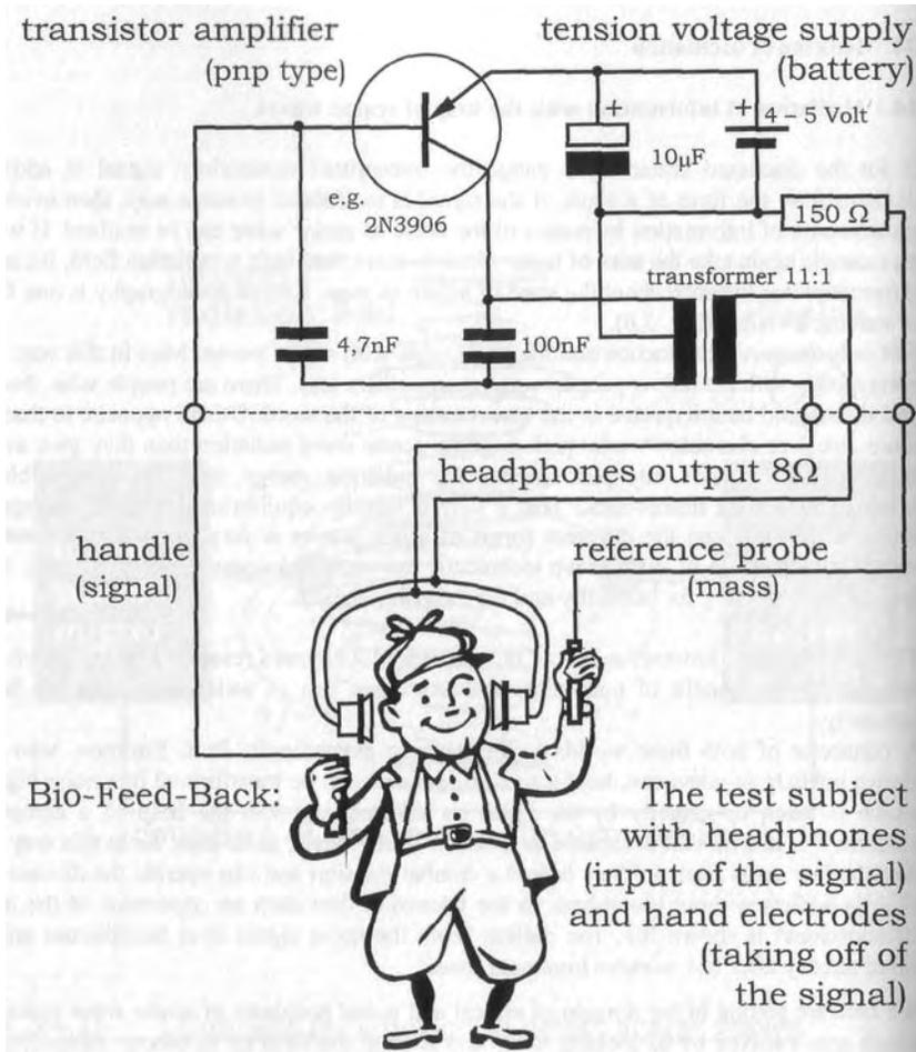
Fig. 24.2 A: Wiring diagram of the Syncrometer. <i>
