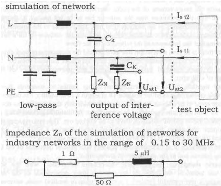
Fig. 2.4: Simulation of network for the measurement of interference voltages.
