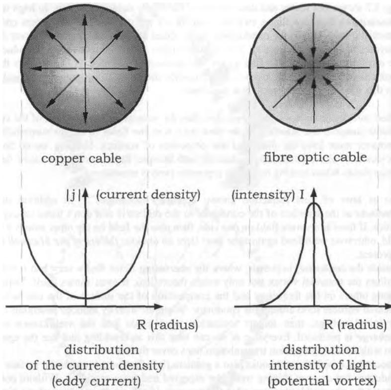
Fig. 4.1: The distribution in principle of the intensity of light within a fibre optic cable compared to the distribution of the current density in a copper cable
