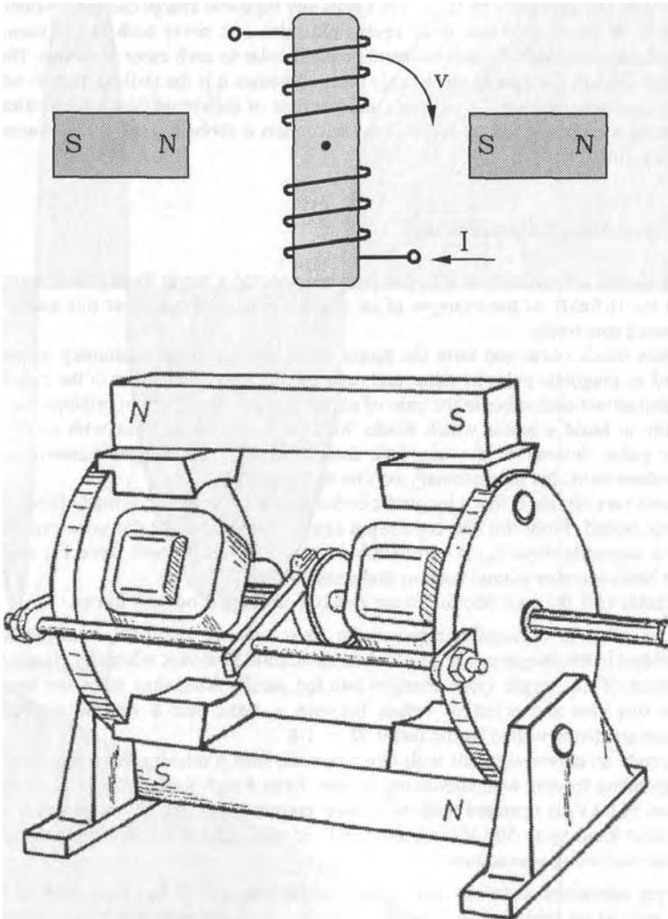
Fig. 15.4: Alternating current dynamo, according to the inventor
