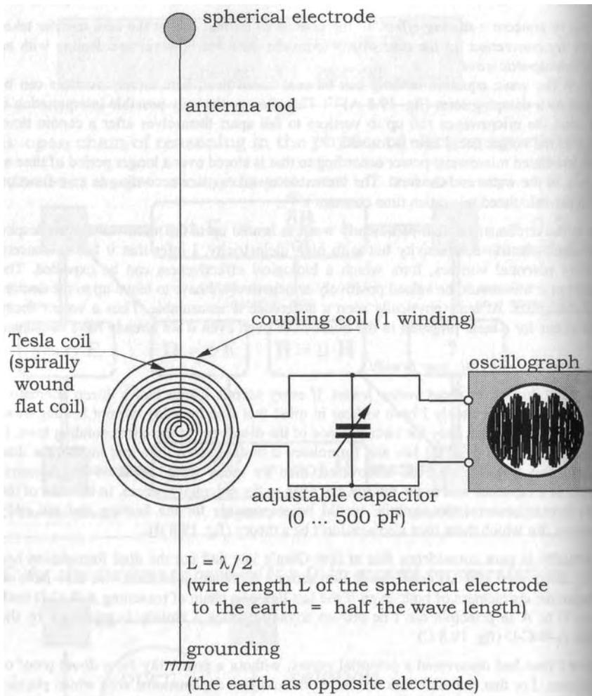
Fig. 19.9: Proof of scalar waves with the Tesla coil.<i>
