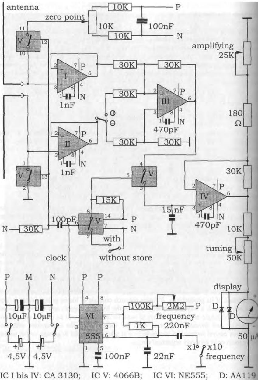
Fig. 19.2: Wiring diagram of the self-built charge amplifier
