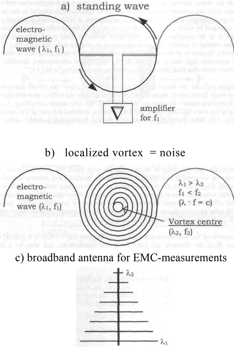
Fig. 1.4: Measurement of localized waves and vortices
