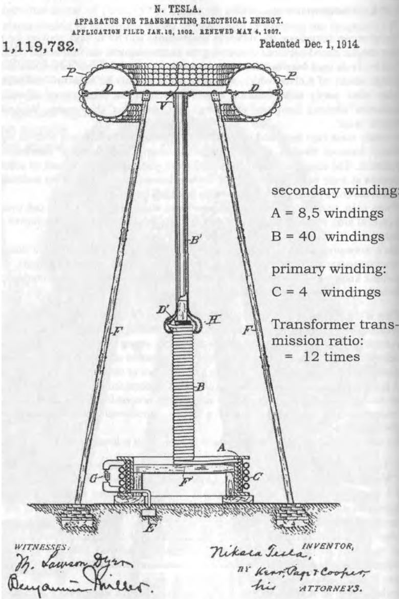
Fig. 9.11: Concerning the technology of the Wardencliff transmitter (fig. 9.10).<sup><i></sup>
