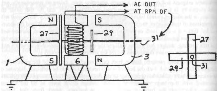
Fig. 16.3: Principle of the Ecklin generator. <i>
