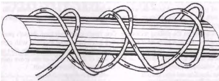
Fig. 16.7 D: Mobius winding arranged like a cross
