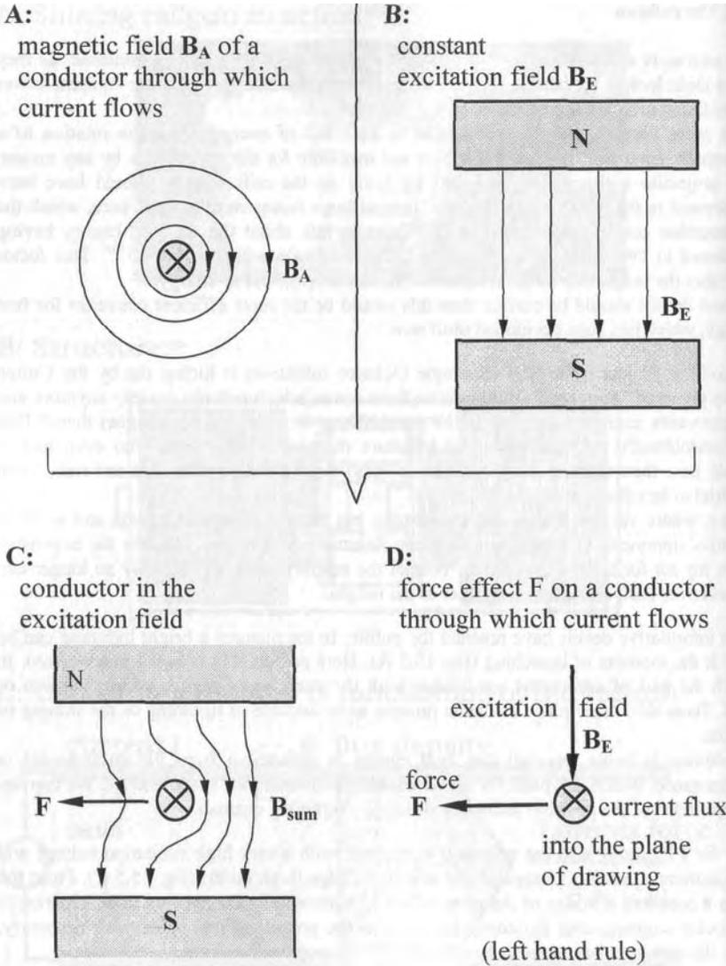
Fig. 15.6: \_\_\_\_\_ The distribution of field lines and force effect on the slider of the railgun through which current flows in a permanent magnetic field
