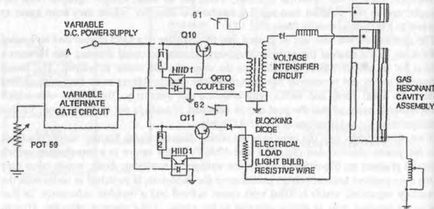
Fig. 17.8: High-tension transformer and driving of the cylindrical water-cell
