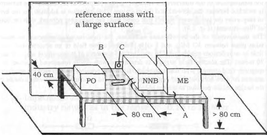
Fig. 2.5: Measurement set up to measure the emission of interferences bound to a conductor,<i>
