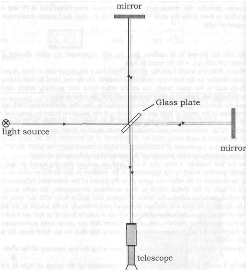
Fig. 6.12: Experiment of Michelson and Morley to detect an aetherwind<sup><i></sup>
