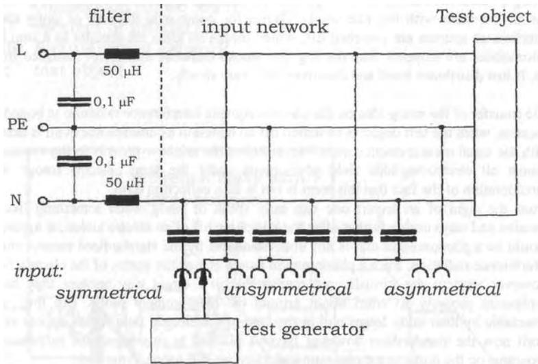
Fig. 2.6: Picking up of interference voltages in network lines. <i>
