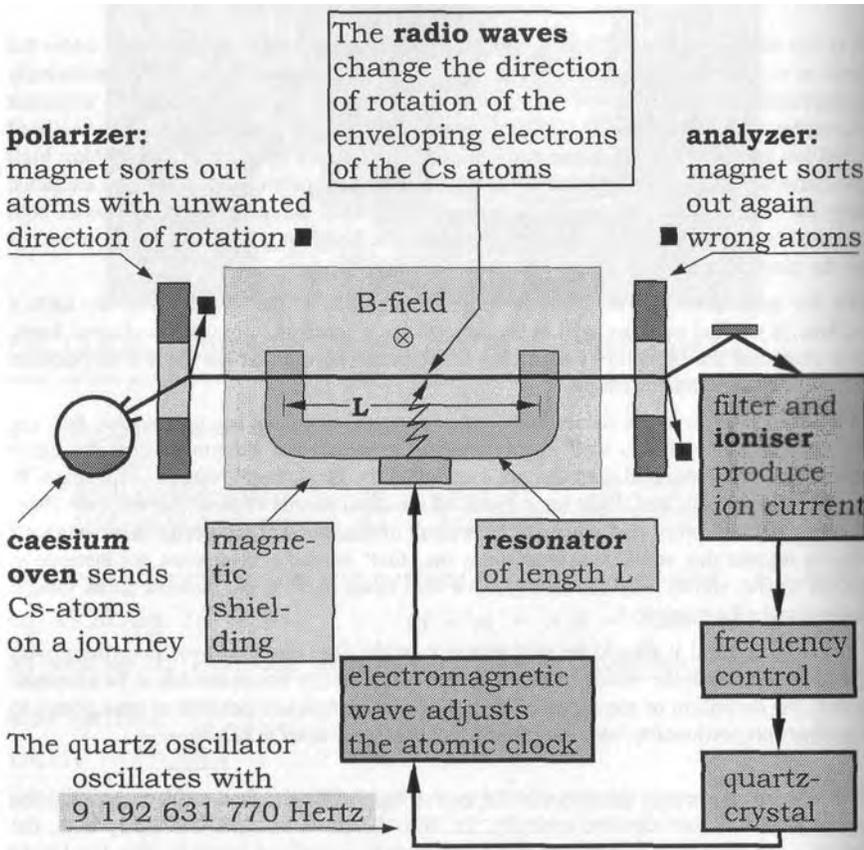
Schematic representation concerning principle of functioning
