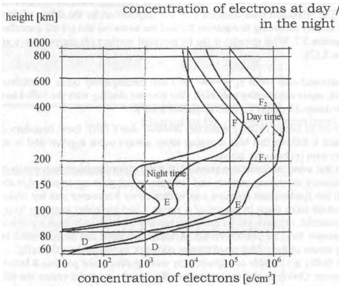
Fig. 5.4: The dependency on height of the ionisation in the ionosphere for medium latitudes . <i>
