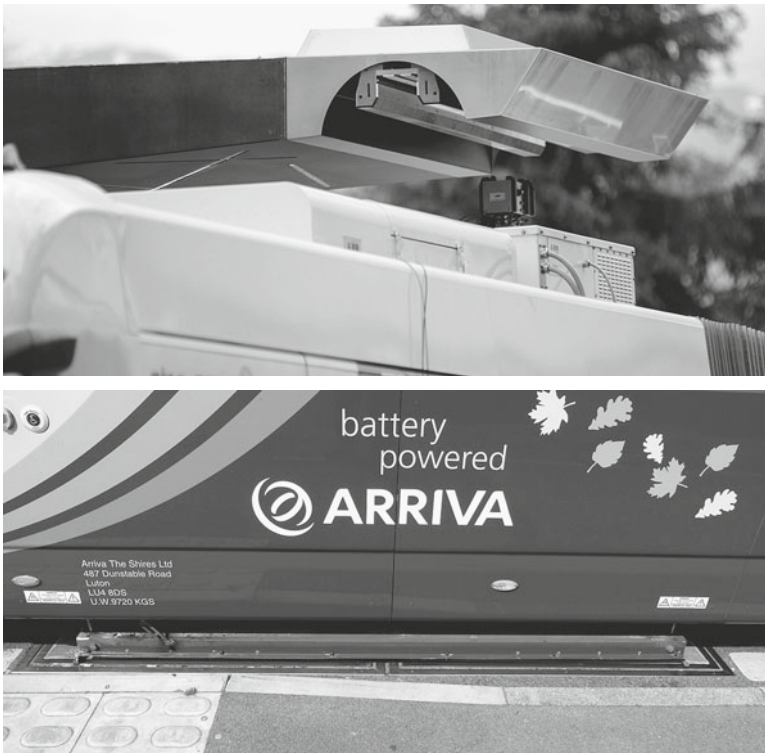
Overhead and undercarriage recharging for electric buses. (Credit, top: Oliver.auge, via Wikimedia commons. Credit, bottom: SpSmiler, via Wikimedia commons.)
