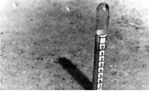
Saccharometer floating in fermenting mash.
