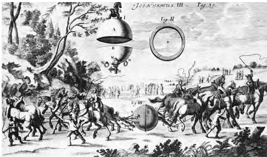
A woodcut, ca. 1850, of Otto Von Guericke's experiment with the Magdeburg Hemisphere demonstrating the pressure of air. © Bettmann/Corbis.
