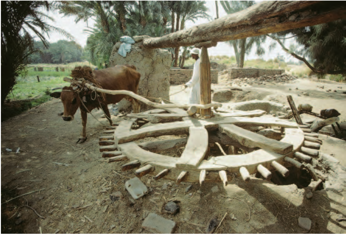
This is a traditional horizontal noria water wheel. The water comes out of the well on a wheel carrying pitchers, which then supplies the irrigation network. © Marc Garanger/Corbis.
