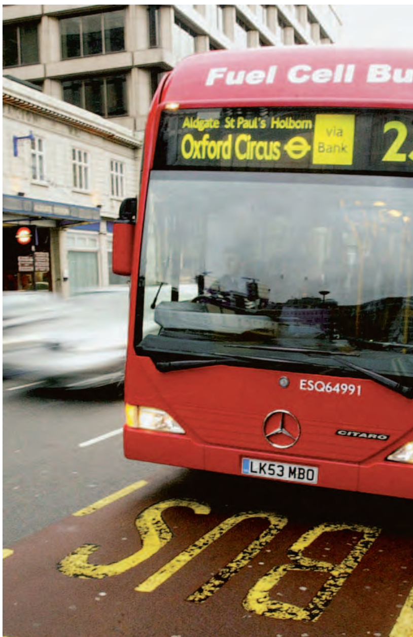
A zero-emission hydrogen fuel cell bus waits at Aldgate bus station on its first day of service in central London, January 14, 2004. The bus emits only water vapor. © Toby Melville/Reuters/Corbis.
