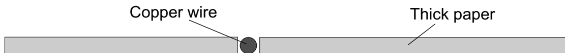
Close up SIDE VIEW of paper slit for PVC slit #2, wire fits in between paper slit.
