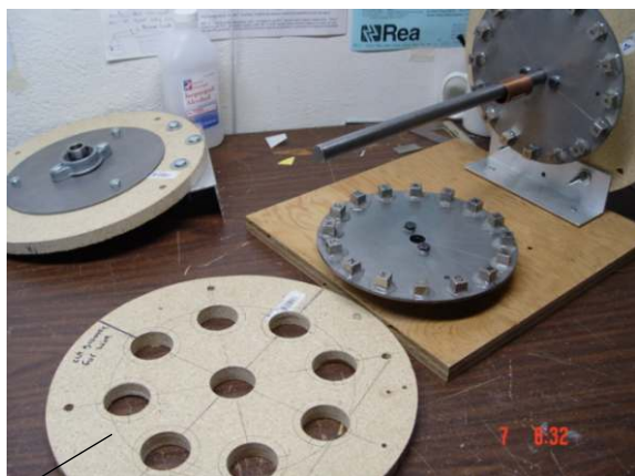
1/2" wood, for holding generator coils
