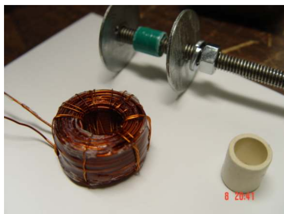
Coil winder removable bobbin. For manual turning on a drill press. Epoxied each layer.
