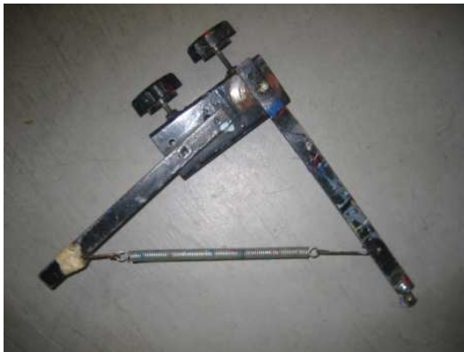
Screen printing Kick leg, Spring loaded, Keeps screen in up position when flooding with ink and lowers
