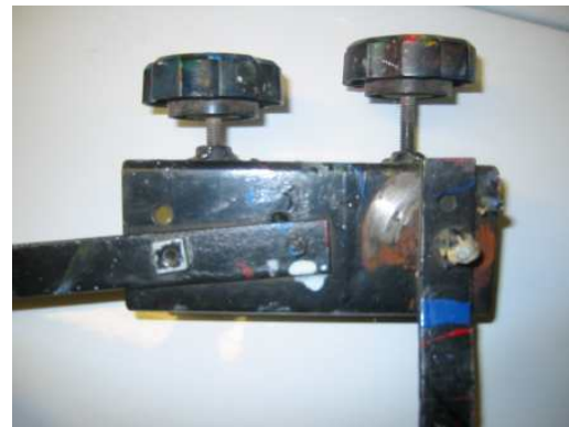
Screen printing Kick leg, Spring loaded, Keeps screen in up position when flooding with ink and lowers
