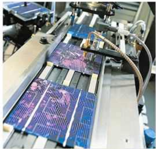
Printing of Photowatt's front-side PV cells.
