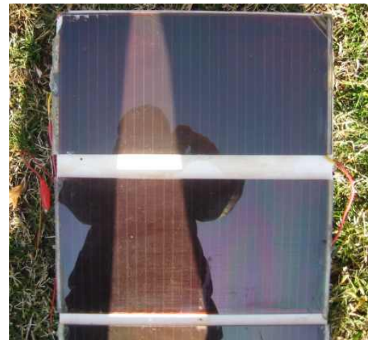
12" x 18" 12 vdc Screen Printed Solar Cells
