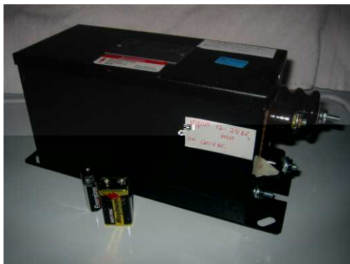
15,000 v Neon Transformer
