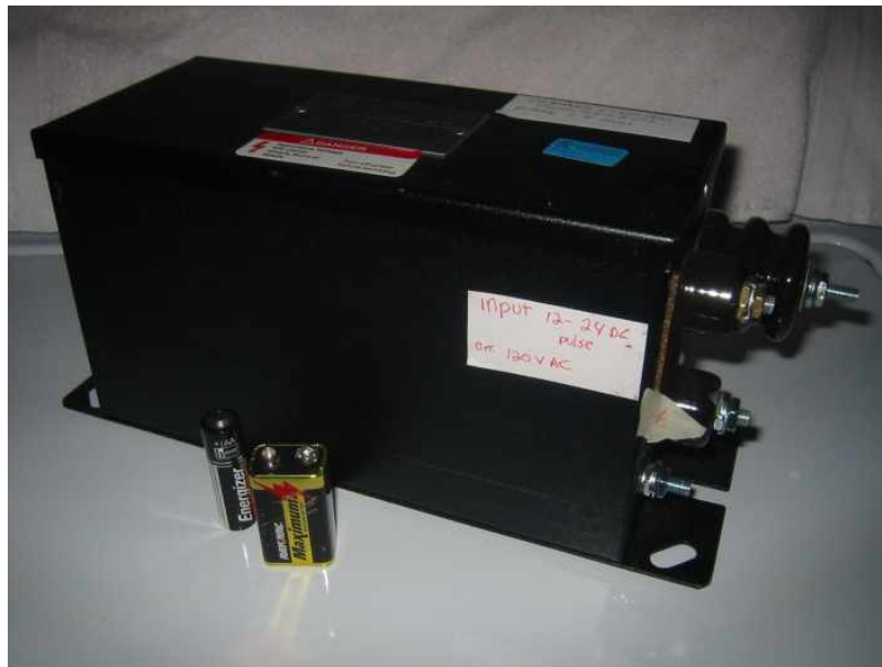
15,000 V Neon Sign Transformer
