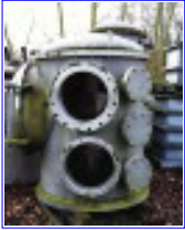
Boeing's stainless steel vacuum chamber proposed for the Podkletnov experiments (Source: Boeing)
