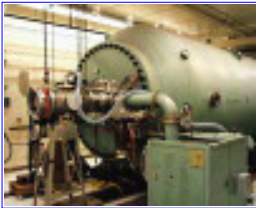
Boeing's Van de Graaff generator proposed for the Podkletnov experiments (Source: Boeing)
