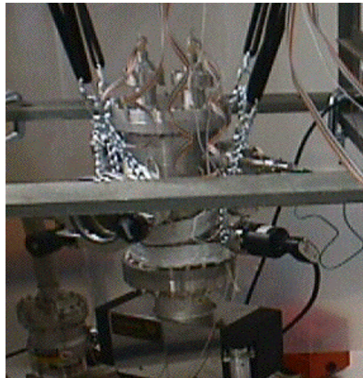
Figure 3. (a) shows the AFM stage below the vacuum flange, connected to the vacuum feedthroughs above. (b) shows the AFM mounted inside a small, stainless steel, vacuum chamber supported by elastic cords to reduce vibration.
