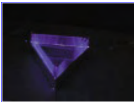
TDT's basic, single triangular cell Lifter photographed using light-enhanced photography shows the device's electrical corona - a side-effect of high-voltage charge transfer
