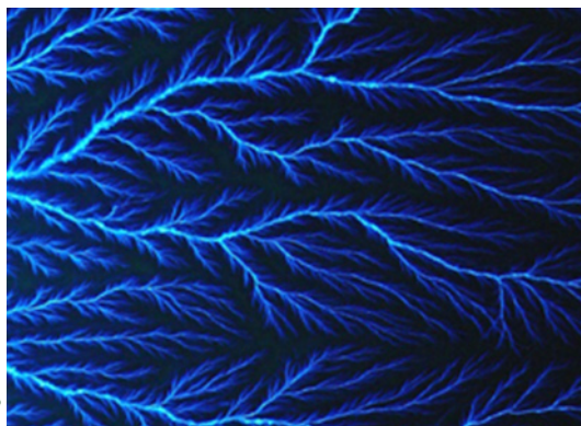
Lichtenberg Figure produced by Electric Discharge ► Credit: Dr John W Gudenas
