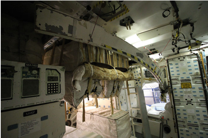
Fig. 4.20 The Space Shuttle's Crew Escape System was a beam to extend from the Shuttle. The crew could use it to escape in case of controlled gliding when unable to land on a runway (Image: B. Ganse)
