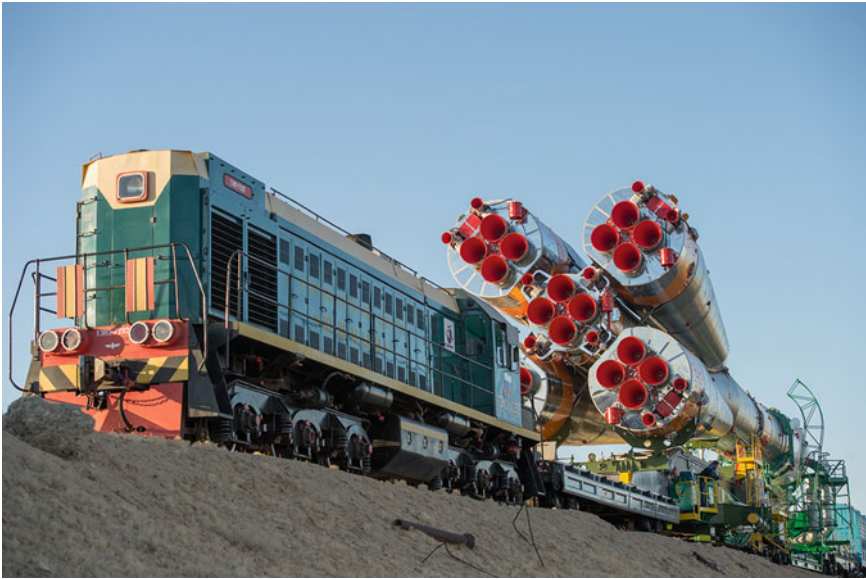
Fig. 3.1 Russian Soyuz rockets are delivered to the launch pad by train and only lifted into vertical orientation once arrived (Image: NASA)
