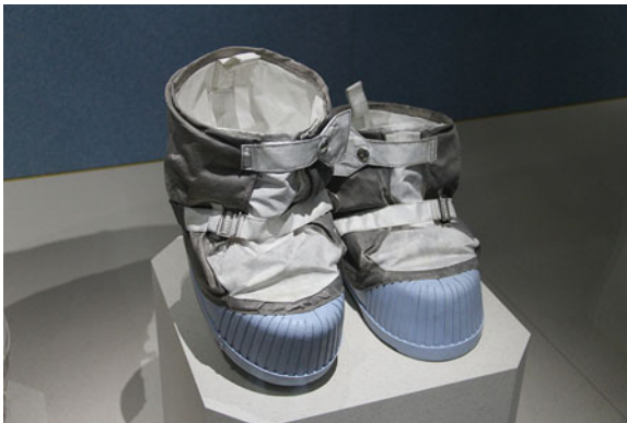
Fig. 4.12 Apollo Moon Boots from 1969 are shoe covers to protect the lunar lander's inside from moondust (Image: B. Ganse)
