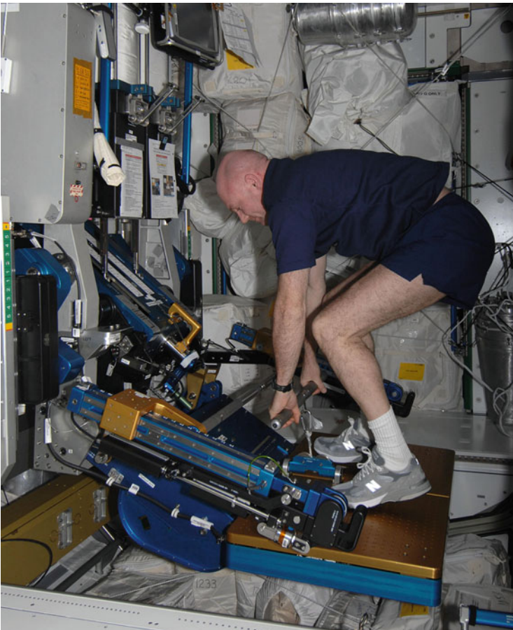
Fig. 5.20 Dutch astronaut André Kuipers using the ARED (Advanced Resistive Exercise Device) on board the ISS (Image: NASA)
