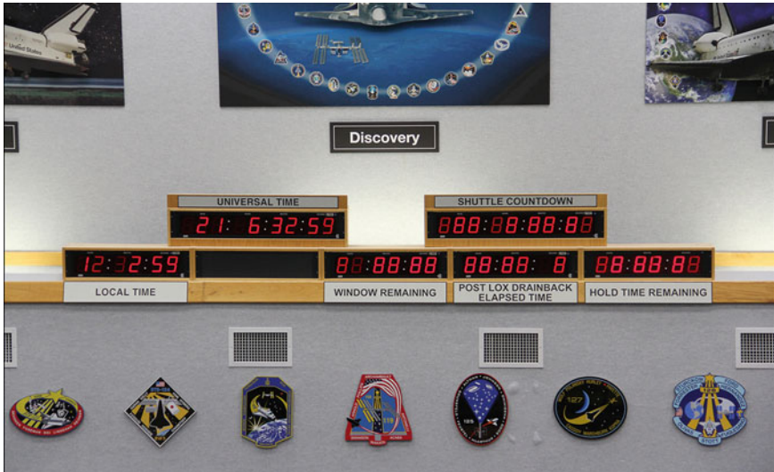
Fig. 3.3 Time displays in the Launch Control Center at the Kennedy Space Center. Universal time = time in days, hours, minutes and seconds since the start of the year. Shuttle countdown = time until launch (T-minus). Local time = time in Florida. Window remaining = time until the launch window closes. Post lox drainback elapsed time = remaining time the spacecraft can stand on the launch pad while filled with liquid oxygen. Hold time remaining = remaining time until the T-countdown continues (Image: B. Ganse)
