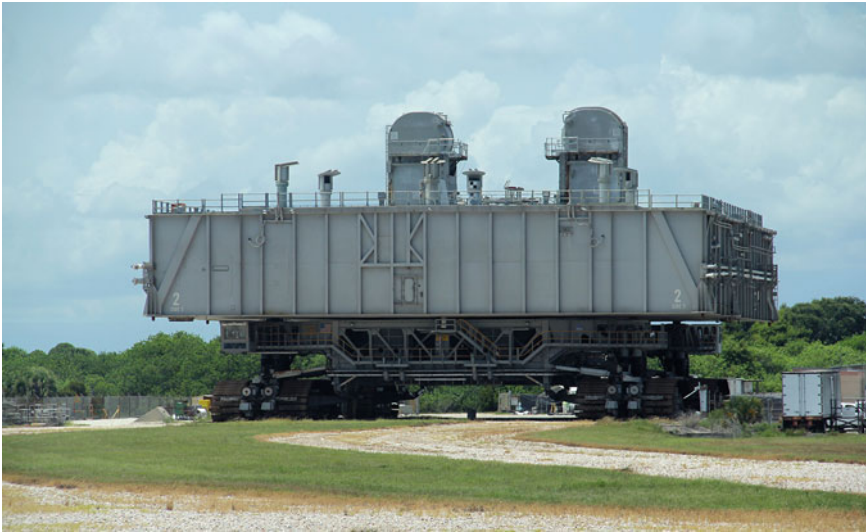
Fig. 2.33 A crawler under a mobile launch platform at the Kennedy Space Center. The crawler is able to carry the entire platform including a rocket to the launch site via the crawlerway (Image: B. Ganse)
