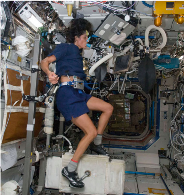
Fig. 5.12 Astronaut Sunita Williams performing a spiroergometry on the cycle ergometer CEVIS on board the ISS (Image: NASA)
