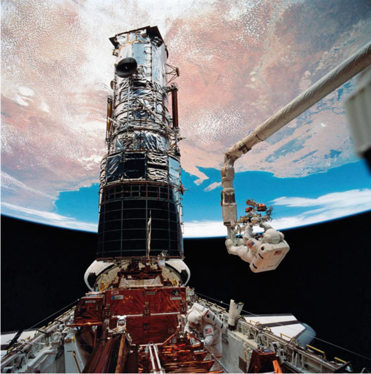
Fig. 5.18 Surgeon and astronaut Story Musgrave repaired the Hubble-Telescope in 1993. The Remote Manipulator System (RMS) carried him to the telescope (Image: NASA)
