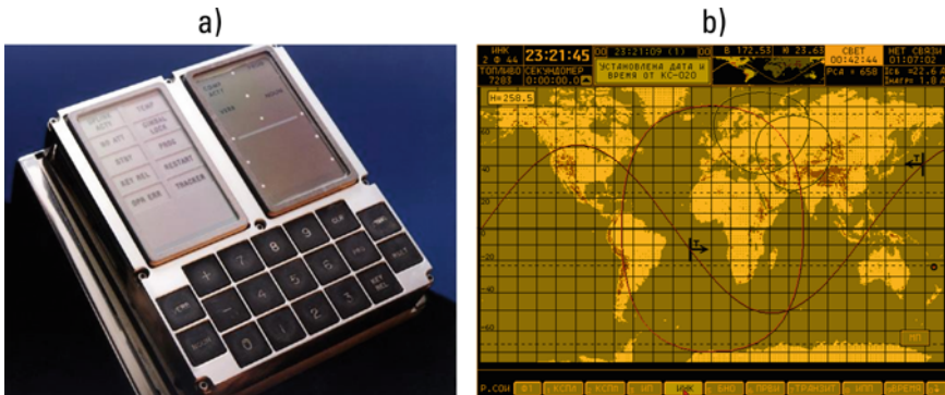
Fig. 2.28 Navigation computers have evolved in the way they display their information. (a) The user interface of the Apollo Guidance Computer only had a small numerical display (Image: NASA). (b) The Soyuz computer software shows a map view with the spacecraft ground track and the Russian radio coverage areas of the ground stations (small misshapen circles over Russia) and a geostationary relay satellite (large red oval) (compare the displays in Fig. 3.6)
