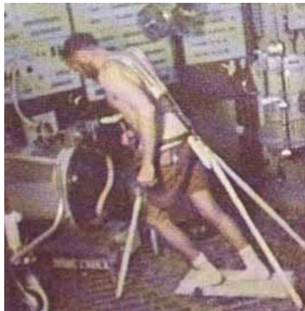
Fig. 5.19 The treadmill on the spacestation Skylab consisted of a Teflon plate and rubber bands. The astronauts had to wear slippery socks to use it, while the rubber bands would pull them towards the Teflon plate. This construction was a milestone in space exercise research (Image: NASA)
