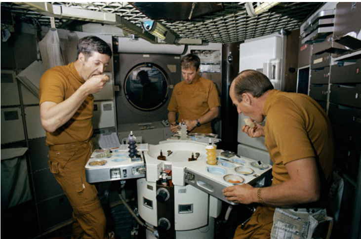
Fig. 2.31 The dinner table of the Skylab spacestation’s ground training facility. A central column can be extended from the floor and food trays can be fixed to the side (Image: NASA)
