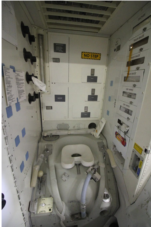
Fig. 2.27 A Space Shuttle toilet (in the Johnson Space Center). Orbital outhouses such as this usually work with vacuum suction (Image: B. Ganse)
