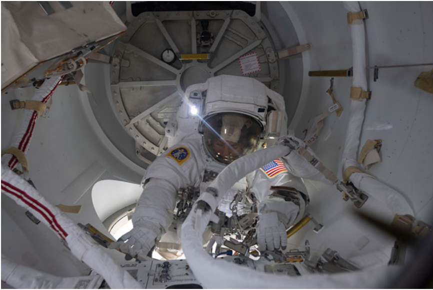
Fig. 5.22 American astronaut Jessica Meir exiting the Quest airlock for her spacewalk of 7 h and 17 min together with Christina Koch in 2019, exchanging a failed battery charge-discharge unit (Image: NASA)
