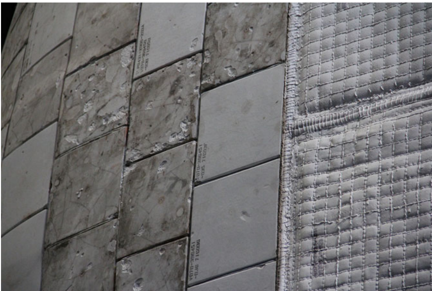
Fig. 2.8 Thermal protection on the side of the Space Shuttle Atlantis. More strongly heated areas are equipped with heat shield tiles, less strongly heated ones are padded with Nomex tissue (Image: B. Ganse)
