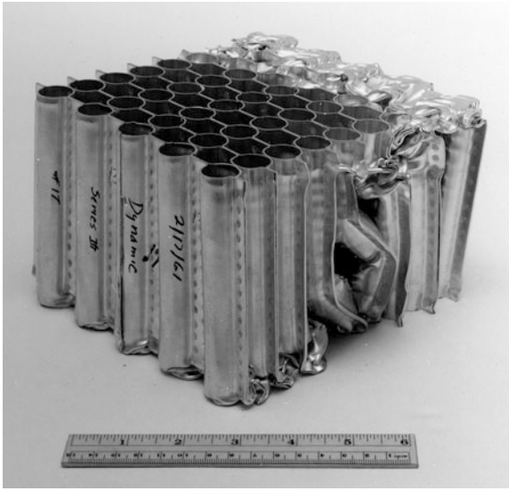
Fig. 2.9 Example of a crush core material, which can absorb kinetic energy by plastically deforming. This specimen was used in the prototype of an uncrewed Surveyor Moon lander (Image: NASA)
