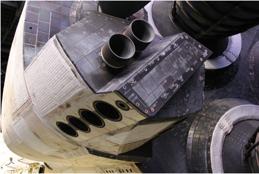
Fig. 2.17 Control thrusters, Vernier rockets and heat shield tiles at the stern of the Space Shuttle Atlantis (Image: B. Ganse)
