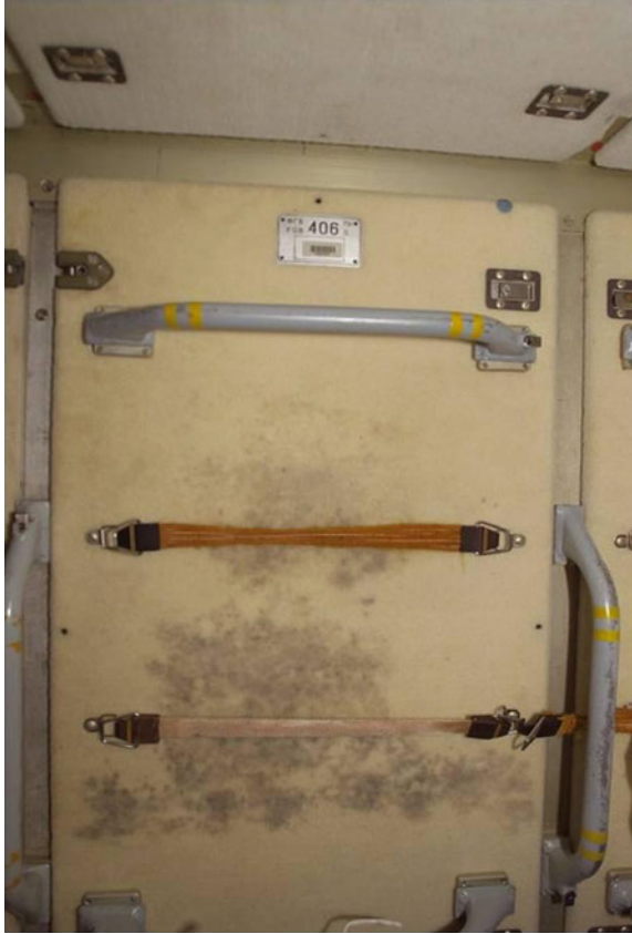
Fig. 4.6 Mould formation on board the ISS on a panel where moist clothing and towels are usually kept to dry (Image: NASA)
