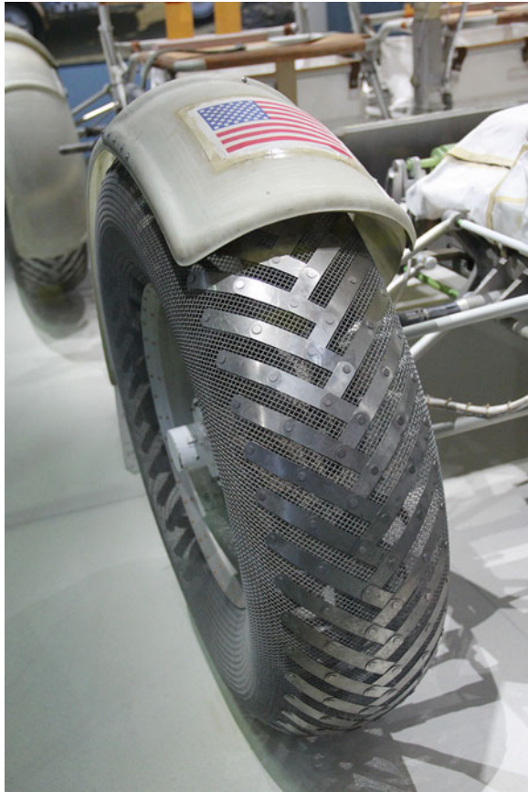
Fig. 6.13 Tire of the Lunar Roving Vehicle in lightweight construction. It was stored on the side of the lunar lander and had to be assembled before use (Image: B. Ganse)
