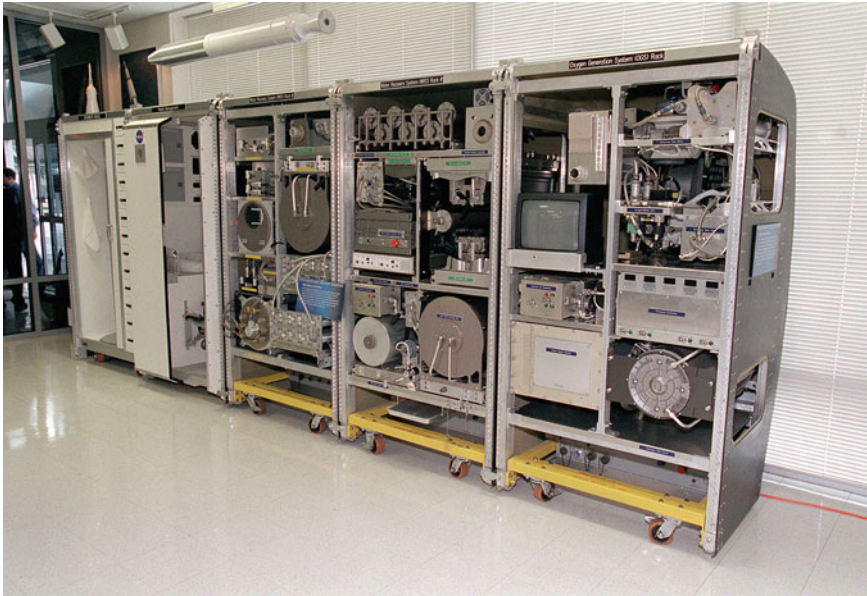
Fig. 2.26 The Environmental Control and Life Support System (ECLSS) of the International Space Station (shown here: a mock-up model on the ground), consisting of oxygen supply, CO 2 removal, air filtration and water processing systems. Each rack is 2 m high and 1 m wide (Image: NASA)
