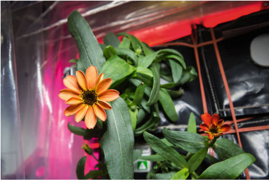
Fig. 6.19 A blooming zinnia in the Veg-01 experiment on the ISS, testing a plant growth system using plant growth pillows (Image: NASA)
