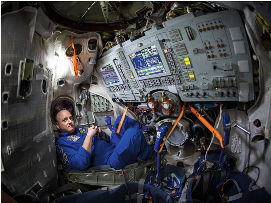
Fig. 3.6 NASA astronaut Scott Kelly in the cockpit of a Soyuz TMA-M capsule. The round object next to the astronaut's knee is a viewing screen, which allows the pilot to look into the direction of the spacecraft's docking port for rendezvous and manoeuvring. The two flight control joysticks are located on both sides of it (Image: NASA)
