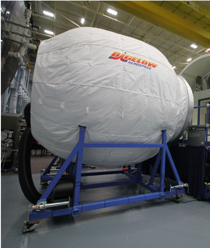
Fig. 6.18 Example of an inflatable spacestation module built by Bigelow Aerospace. The photo was taken in building 9 of the Johnson Space Center (Image: B. Ganse)
