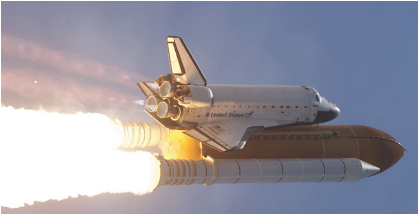
Fig. 2.16 Mach diamonds are visible in the exhaust plume of the Space Shuttle Main Engines (SSME) at the back of the orbiter. In these spots, shock waves focus within the engine exhaust. Since the engines are in use throughout the whole extent of the atmosphere, they are slightly overexpanded for low altitudes (Image: NASA)
