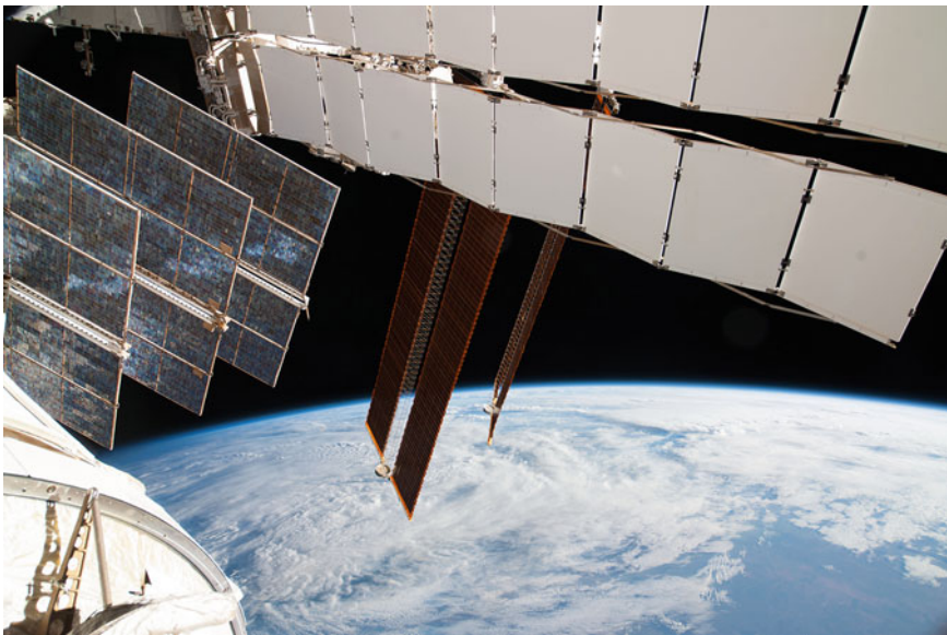
Fig. 2.24 Cooling panels (white) on the International Space Station. The ammonia coolant cycle of the station flows through these panels which radiate heat out into space as infrared radiation (Image: NASA)
