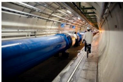
▲ At the LHC beams are accelerated inside tubes 27 km long in tunnels.
