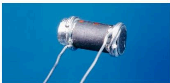
▲ A thermistor and its circuit symbol.
