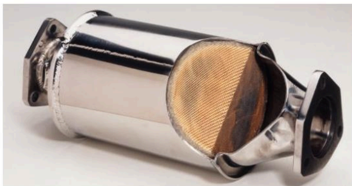
▲ The honeycomb structure of a catalytic converter.
