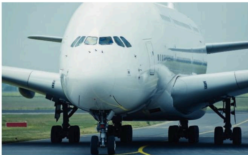
▲ The world's largest passenger aeroplane, the Airbus A380, is made from composite materials.
