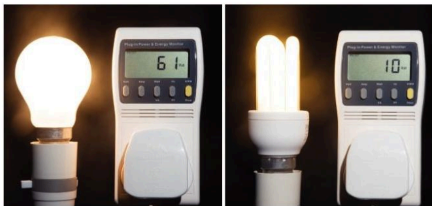
▲ The bulbs are the same brightness but the one on the right has a much lower power.
