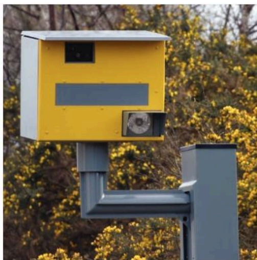
▲ A speed camera measures how long it takes a car to travel a certain distance by taking a photo at the start of the distance and another at the end. It can then calculate the car's speed.
