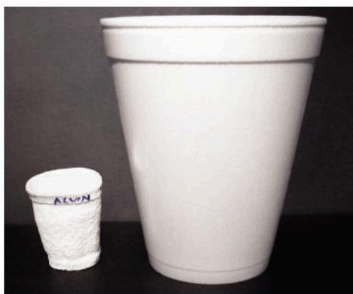
▲ The cup on the left was taken down to a depth of 3000 m.
