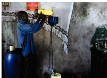
▲ This is a LifeStraw. It contains hollow fibres. The fibres filter the water, removing bacteria and parasites.
