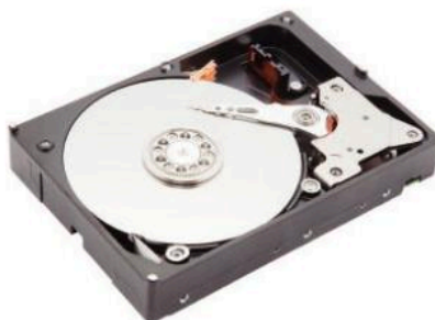
▲ A hard disk. This stores data on a computer.
