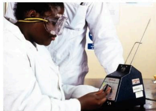
▲ Apparatus used to measure melting points.
