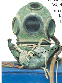
A stone was used to weigh divers to keep them near to the seabed.
