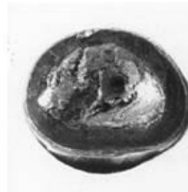
Base of bullet CE 399, showing minor distortion and area where some metal was missing. (Removed for laboratory analysis.)
