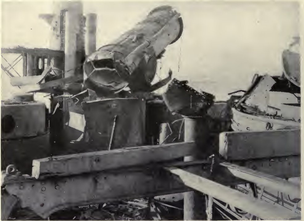
THE WHOLE CENTER PART OF THE "INDIANA" WAS SMASHED TO PIECES BY ONE AËRIAL BOMB WHICH WAS PLACED ON DÉCK AND DETONATED
