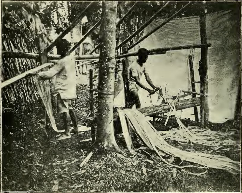
THE BAST STRIPS OF THE MUSA TEXTILIS AFTER BEING DRAWN SEVERAL TIMES UNDER THE KNIFE
