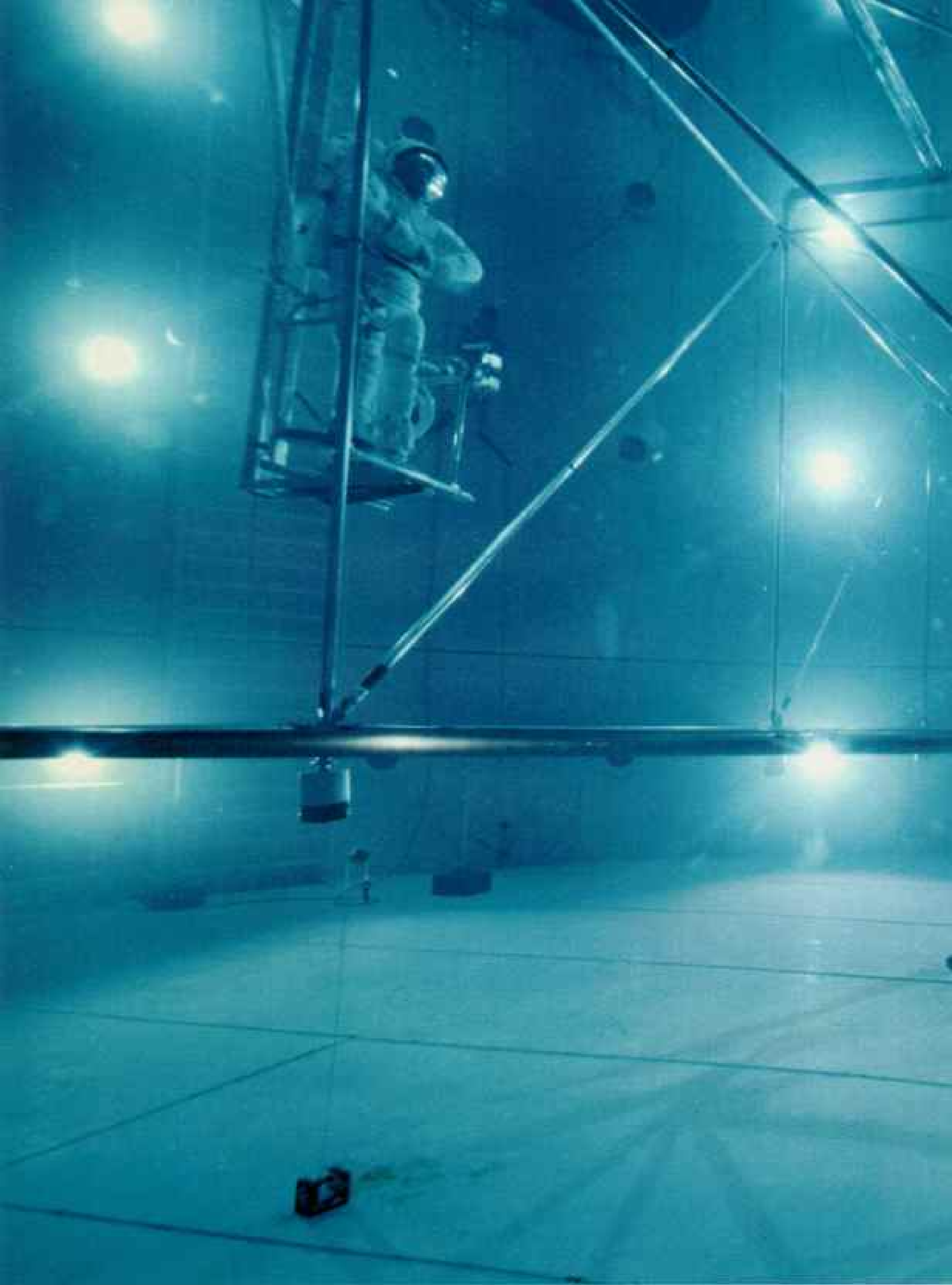
Simulating weightlessness in a 40-foot-deep water tank, space-suited NASA engineers at Huntsville, Alabama, test hardware designs and assembly procedures by building the primary framework for the planned U. S. space
