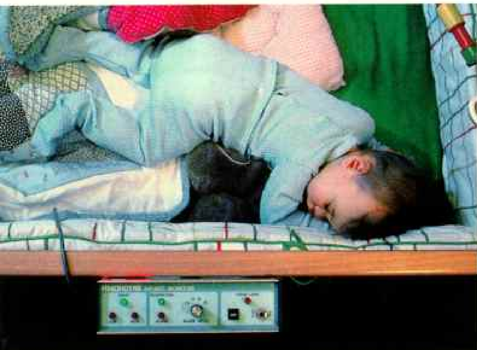
ELECTRONIC SENTRIES guard against sudden infant death syndrome (SIDS), a mysterious phenomenon that strikes mostly during sleep. In the United States SIDS is the leading cause of death from one month to one year of age. Electrodes beneath the pajamas of a seven-month-old (above) whose brother died of SIDS lead to a home monitor that detects abnormalities in pulse or respiration. At Massachusetts General Hospital in Boston, a host of functions are tracked on an infant victim (opposite) of severe apnea, the intermittent cessation of breathing.
