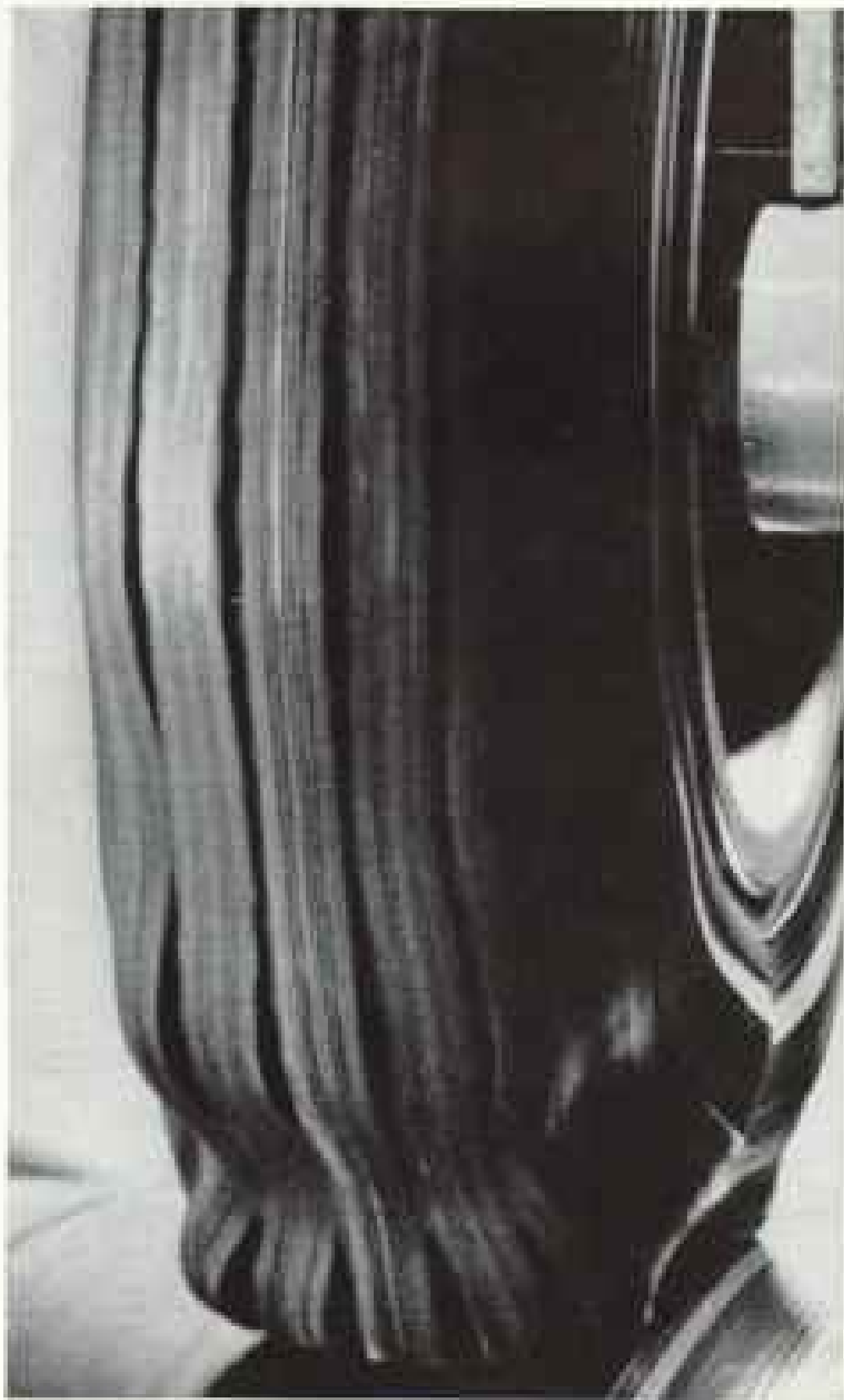
This is squirm at high speed. We ran this conventional two-ply tire in our laboratories at exaggerated speeds (under rated conditions) so you can see how bad tread squirm can get. Notice how the tread surface of this two-ply tire is badly distorted.
