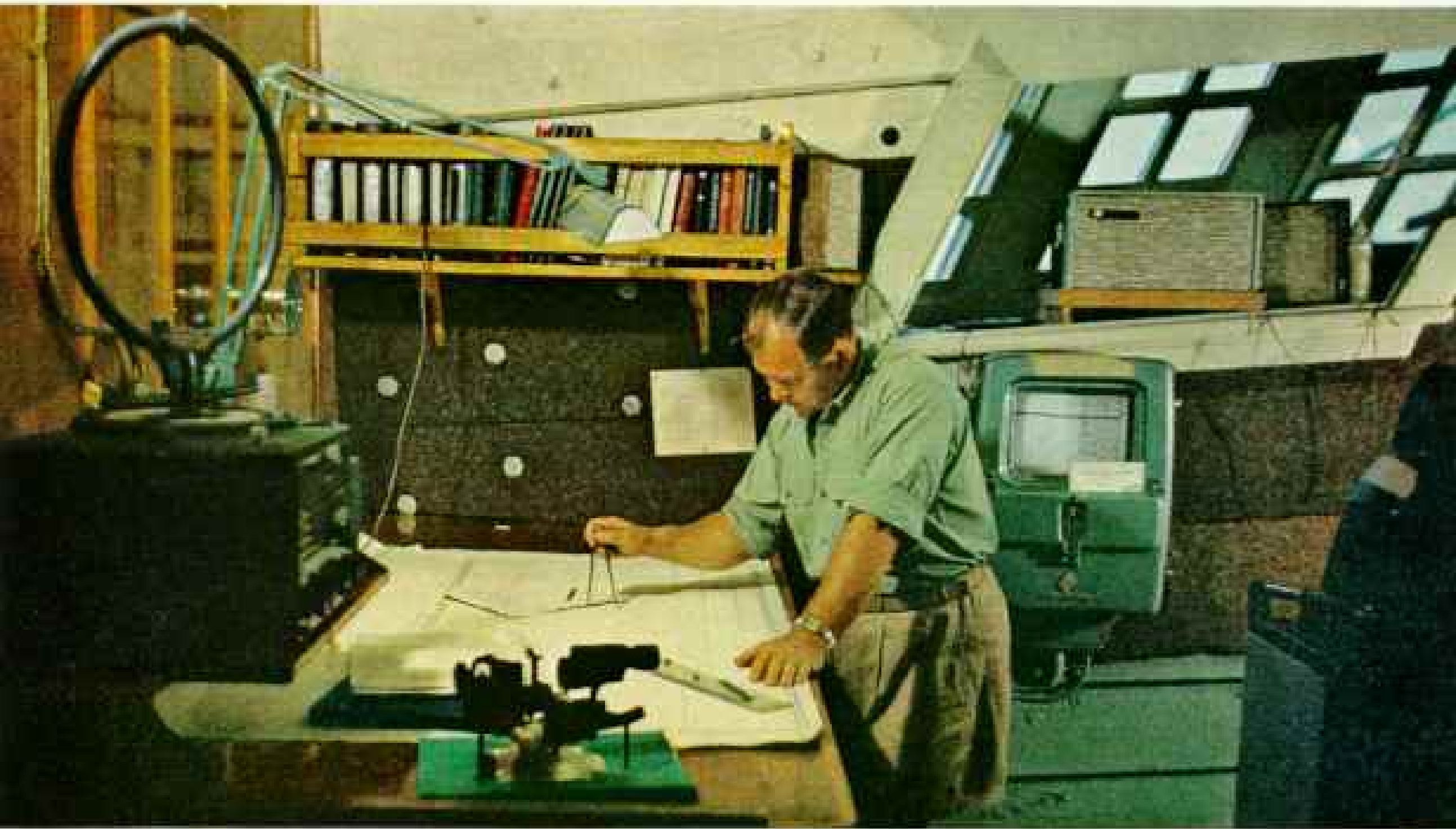
"I have determined the Longitude": Bligh's log. Capt. Ellsworth Coggins, master of Bounty , plots his position. Behind him, the depth indicator; at left, the loop of the radio direction finder. Plath sextant stands on the chart table.
