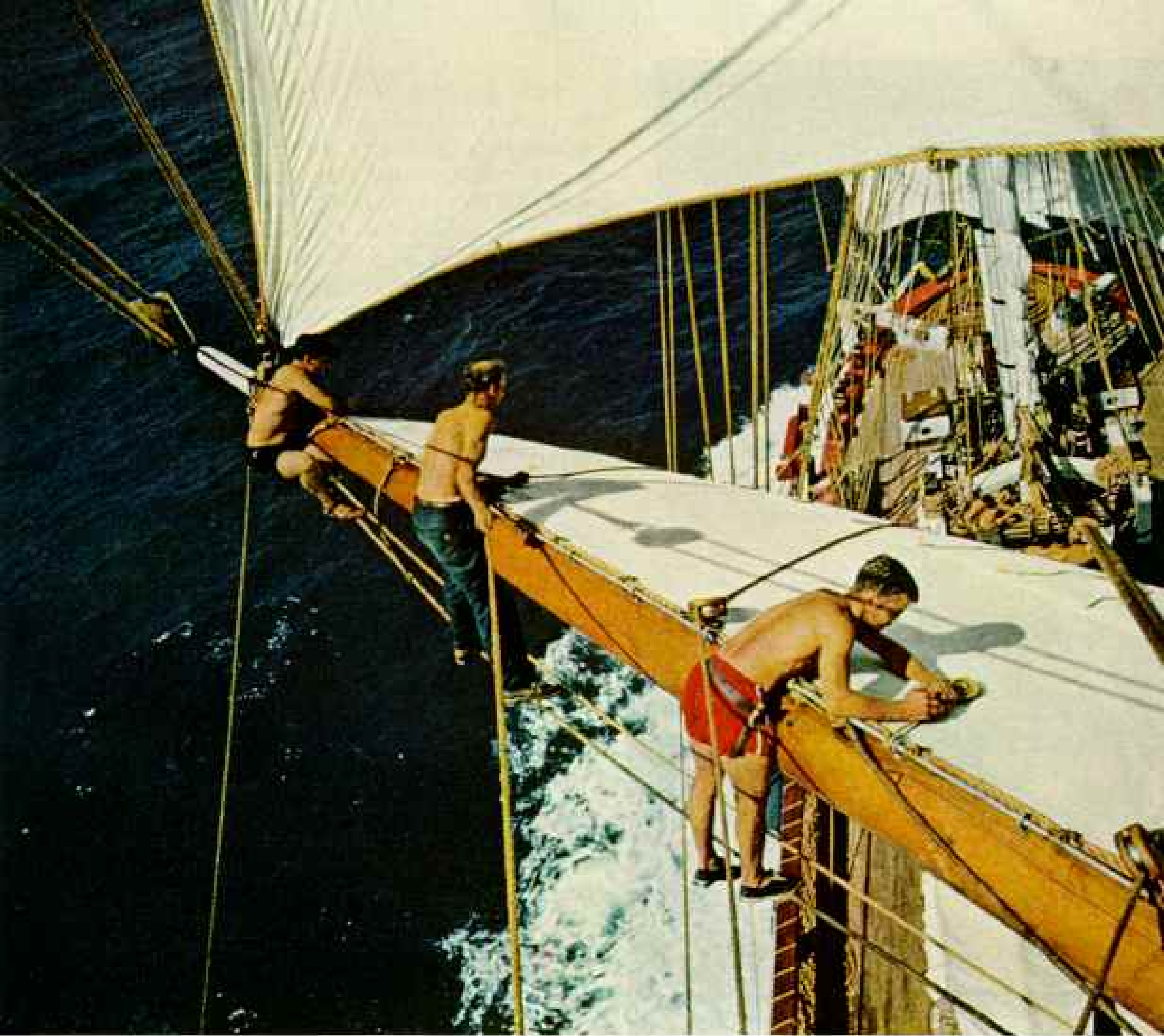
"All Sails set." Crewmen make up the mainsail gaskets as Bountey scuds at 10 knots
