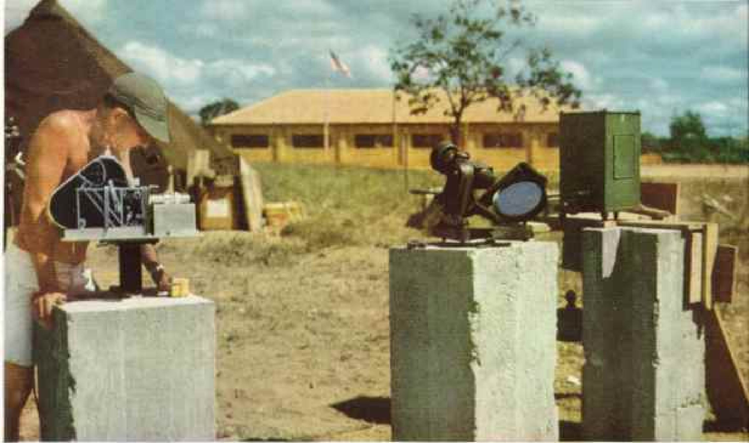
His Camera Photographs the Eclipse Reflected in a Mirror that Follows the Sun In this way Staff Photographer R. H. Stewart obtained clear, steady motion pictures. Note sky reflection in mirror.
