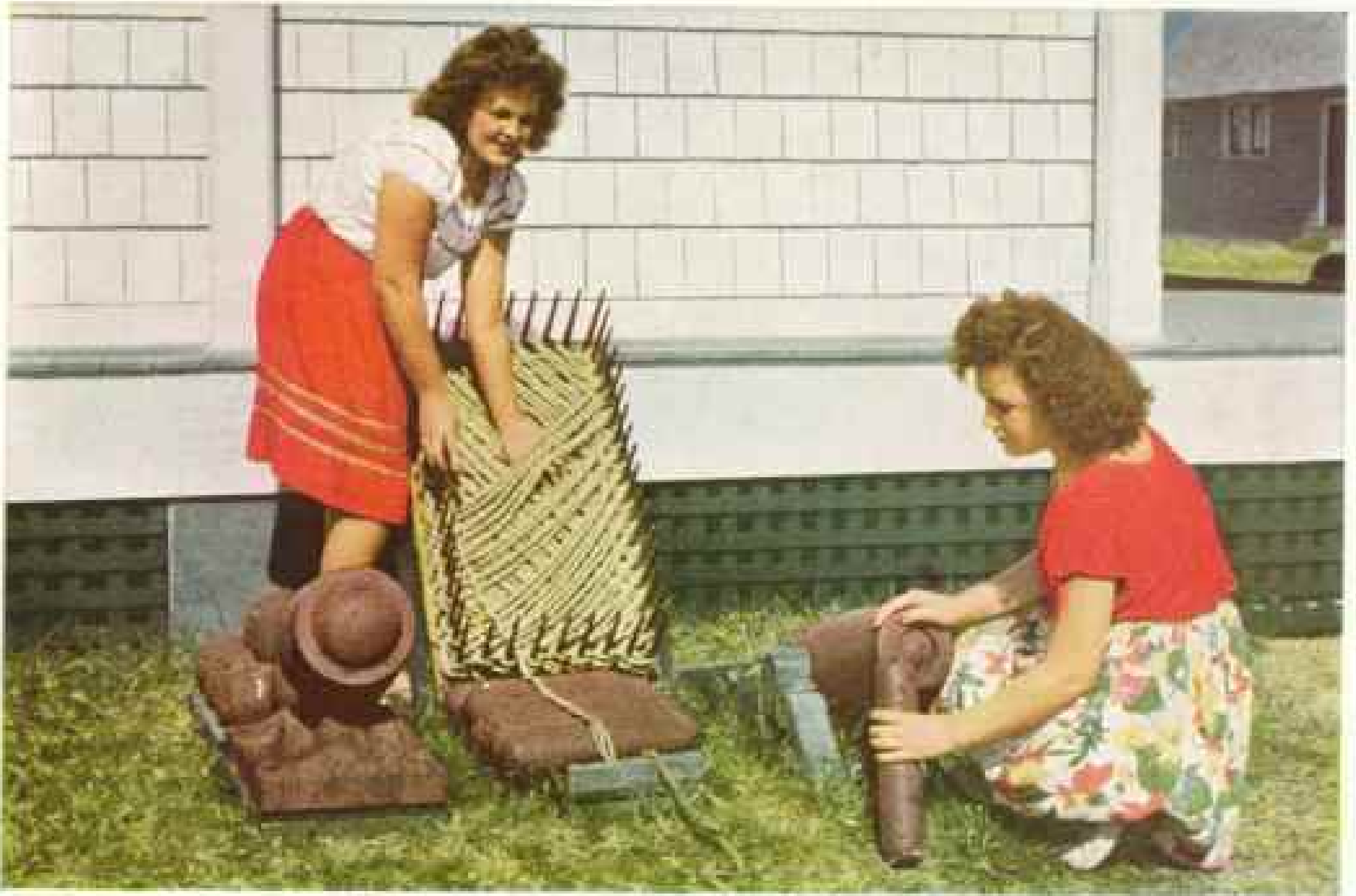
These Old Mortars Shot Many a Life Line to Vessels Wrecked Near Caffey's Inlet Before a gun was fired the pegs were removed from the "faking box," thus clearing the line for easy running. Modern Lyle gun and paillike container for line replace this old equipment.
