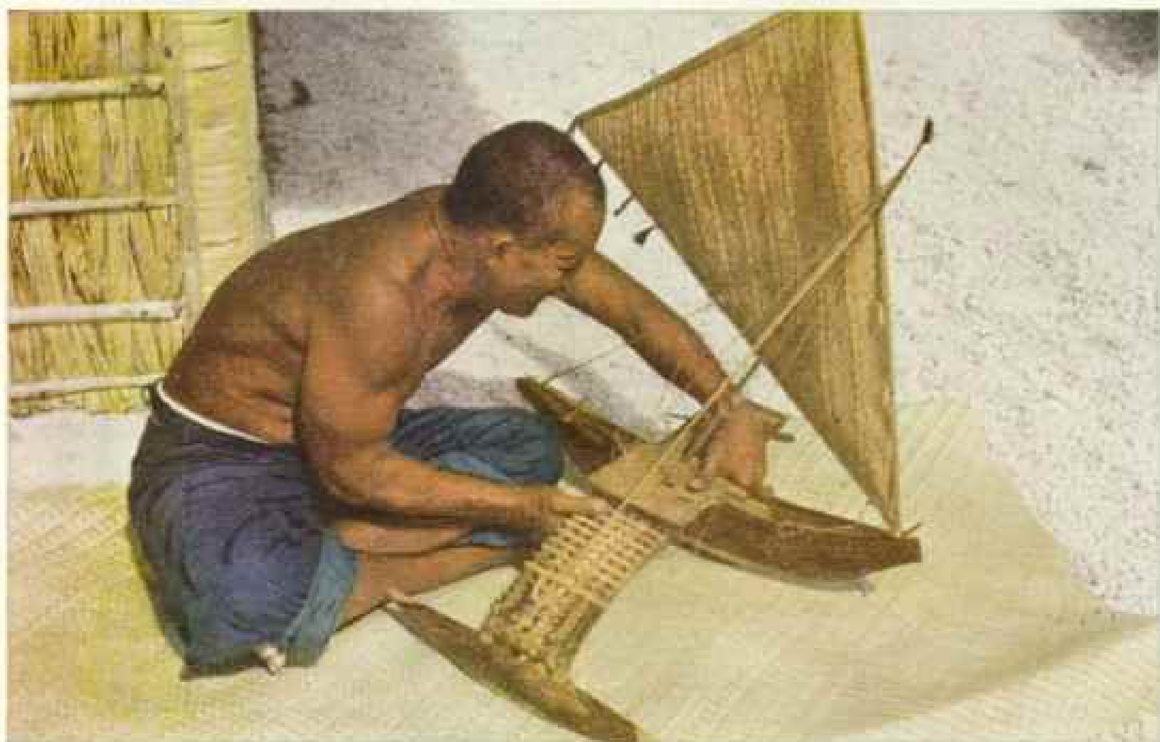
Deftly He Finishes a Model, Lashing Hull and Outrigger Together with Coconut-fiber Twine One of the best canoe builders in Kwajalein Atoll, this Marshallese has constructed many full-sized native craft.
