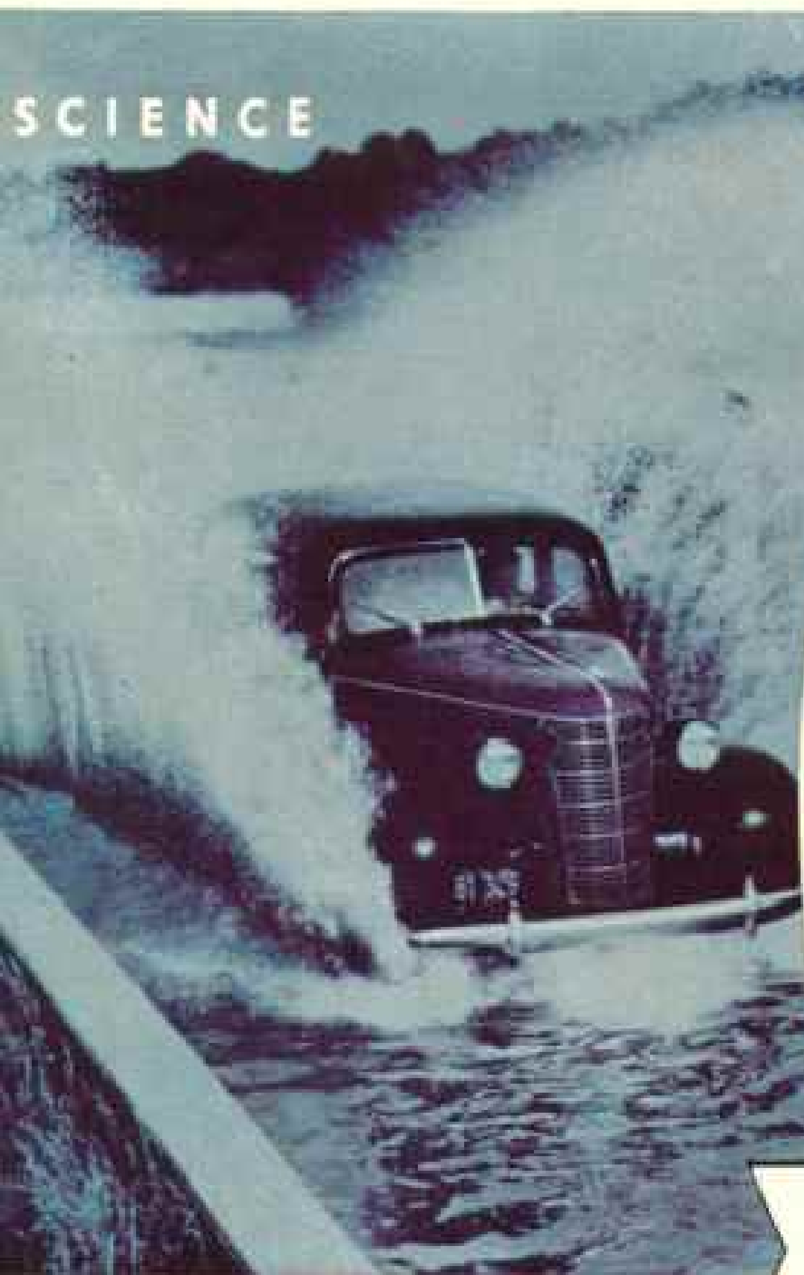
THE "BATHTUB" is the General Motors proving ground — only one among scores of tests used to check engineering features on new cars.
