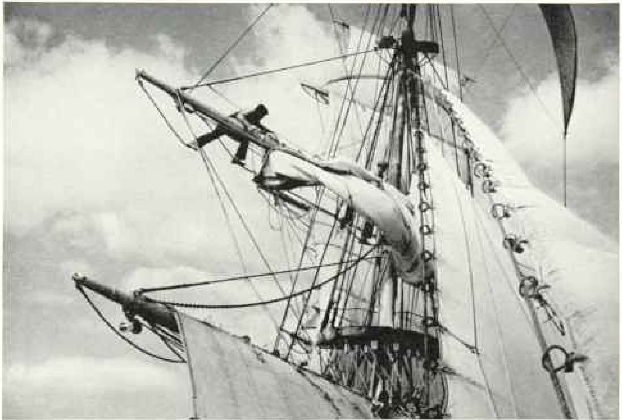
TWO DAYS ARE REQUIRED TO CHANGE A SHIP'S HEAVY CANVAS TO A LIGHT SUIT
