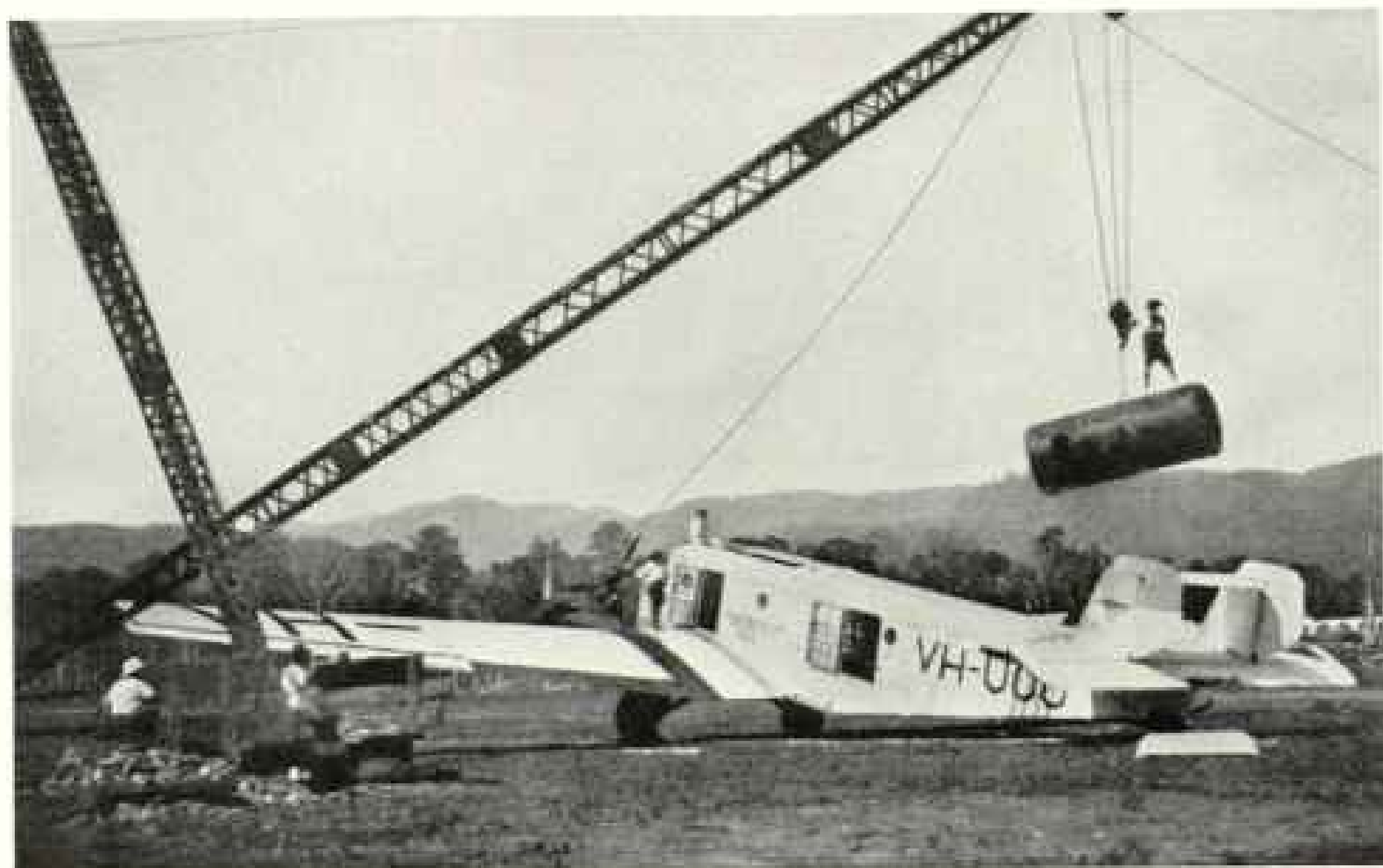
THE AIRPLANE EXPRESS UNLOADS A THREE-TON BOILER AT THE BULOLO GOLD FIELDS, IN NEW GUINEA.
