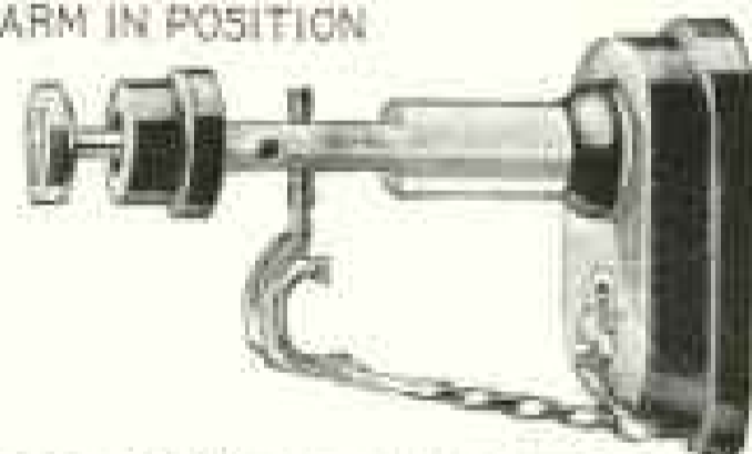
MOTOR STOPPED, EXPANSION OCCURRING IN THERMOSTATIC ARM, WHICH IS JUST ABOUT TO RELEASE PLUNGER
