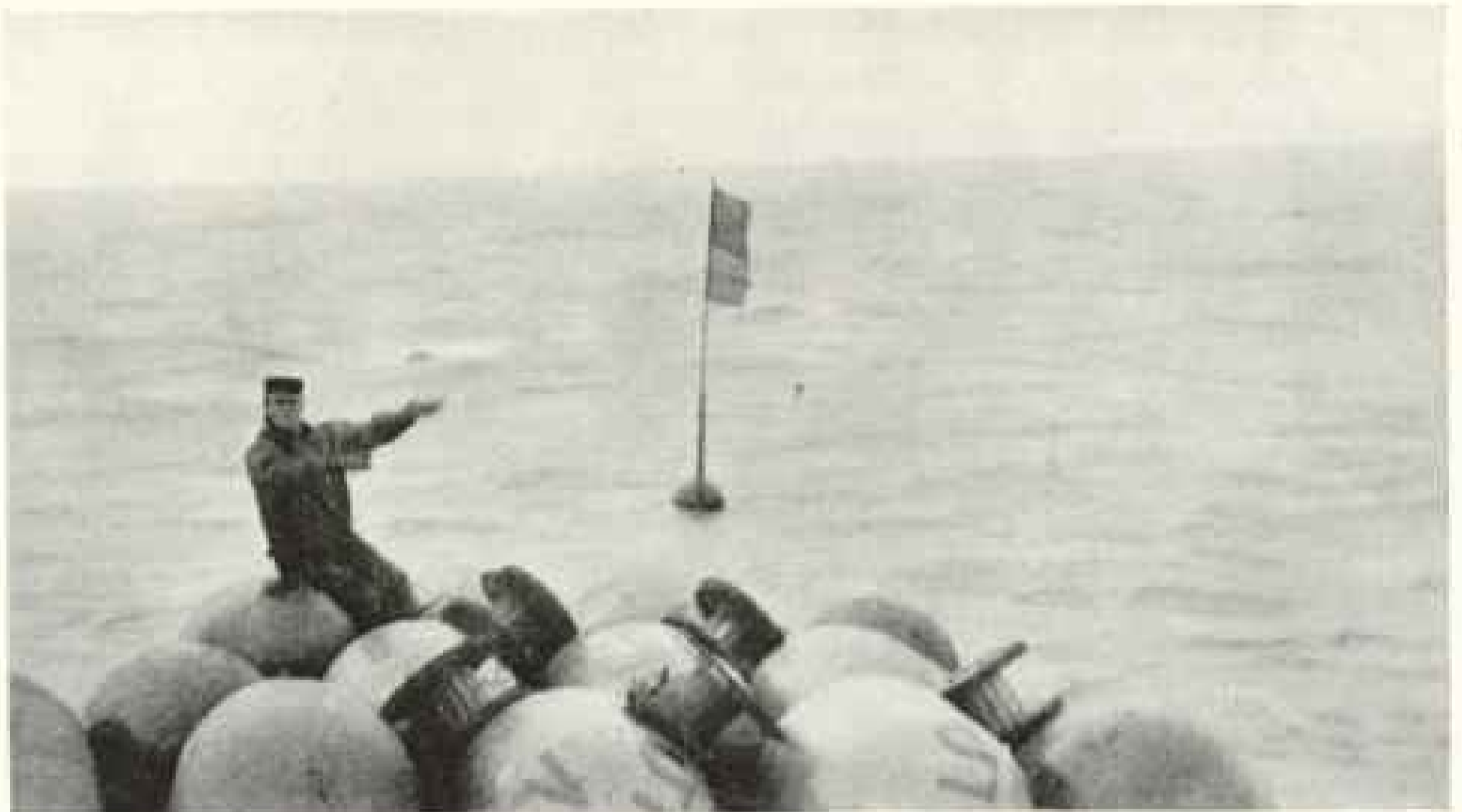
MARKER BUOYS TO INDICATE THE POSITIONS OF THE LINES OF MINES WERE PLACED AT INTERVALS OF THREE MILES THROUGHOUT THE LENGTH OF EACH GROUP
