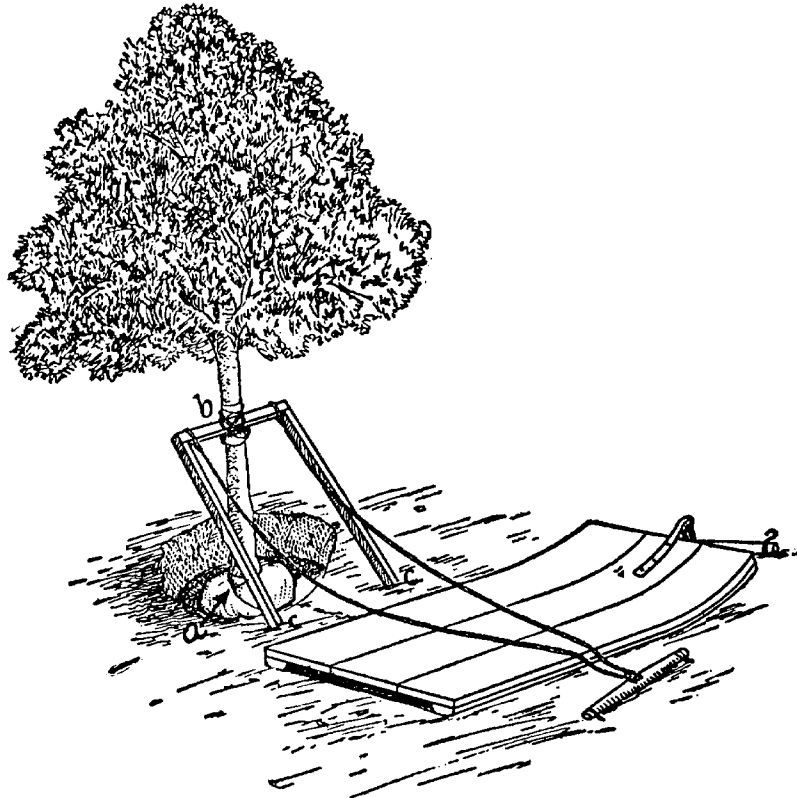
RIG FOR MOVING TREE
