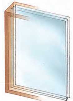
Windows are triple-glazed to keep out the cold. The air between the three layers of glass acts as insulation.
