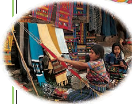
Weavers use a backstrap loom that can be moved from place to place.
