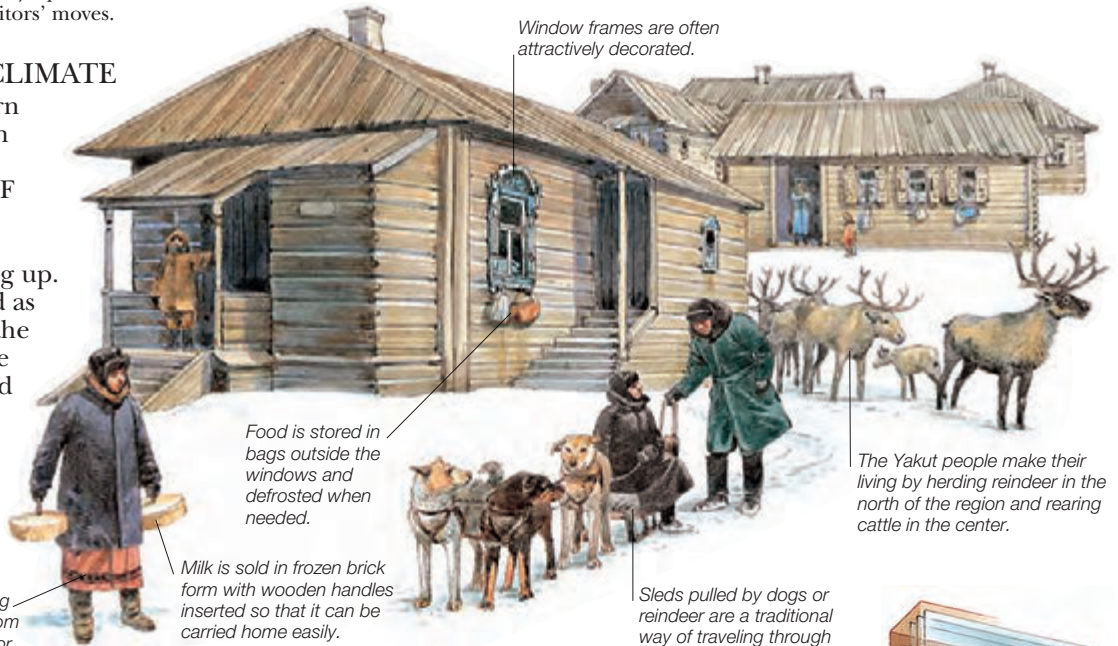
Windows are triple-glazed to keep out the cold. The air between the three layers of glass acts as insulation.
