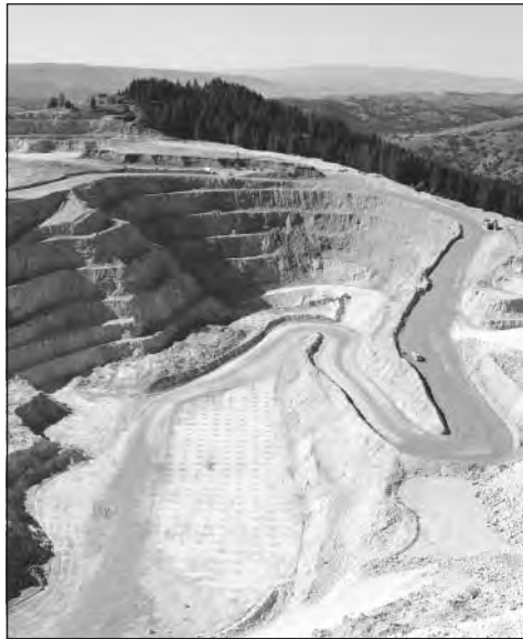
Strip mining involves the removal of long narrow strips of surface materials, using excavation equipment called draglines, so that underlying minerals can be collected easily. (PhotoDisc)
