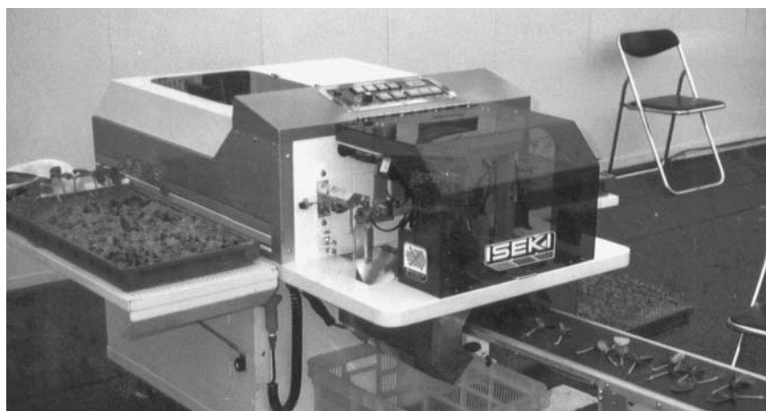
Figure II.C.6.11. In Japan, watermelon seedlings are grafted by machine onto Fusarium-resistant rootstocks.
