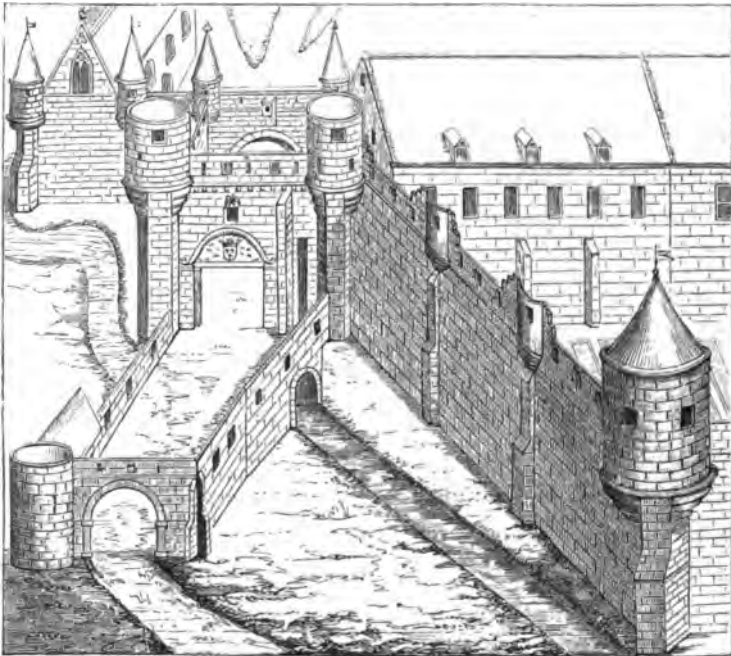
Fig. 251.—Saint-Jean des Vignes, an Abbey of Regular Canons at Soissons (1076), the entrance-gate guarded by a barbican and bastilles.—From an Engraving in vol. i. of "Architecture Monastique," by M. Albert Lenoir.
