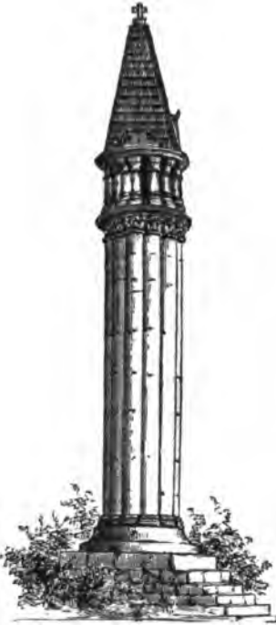
Fig. 394.—Beacon in the Cemetery of Feniou, near St. Jeand'Angely (Eleventh Century); it is formed of eleven Roman columns.
