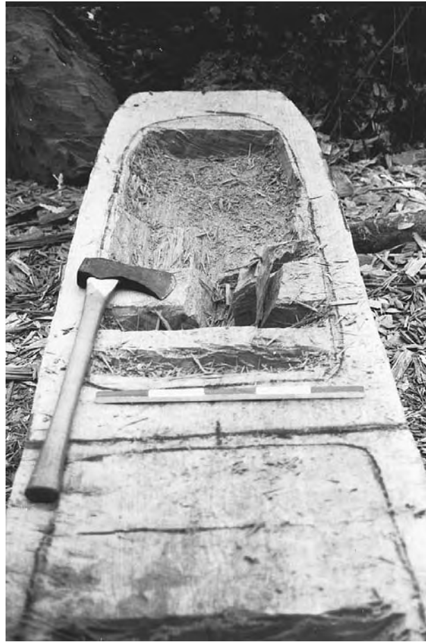
Fig. 1. Replica of the Clapton tenth-century Anglo-Saxon dugout boat being hollowed out by an axe as dictated by the toolmarks found on the original. COURTESY OF D. M. GOODBURN. REPRODUCED BY PERMISSION.
