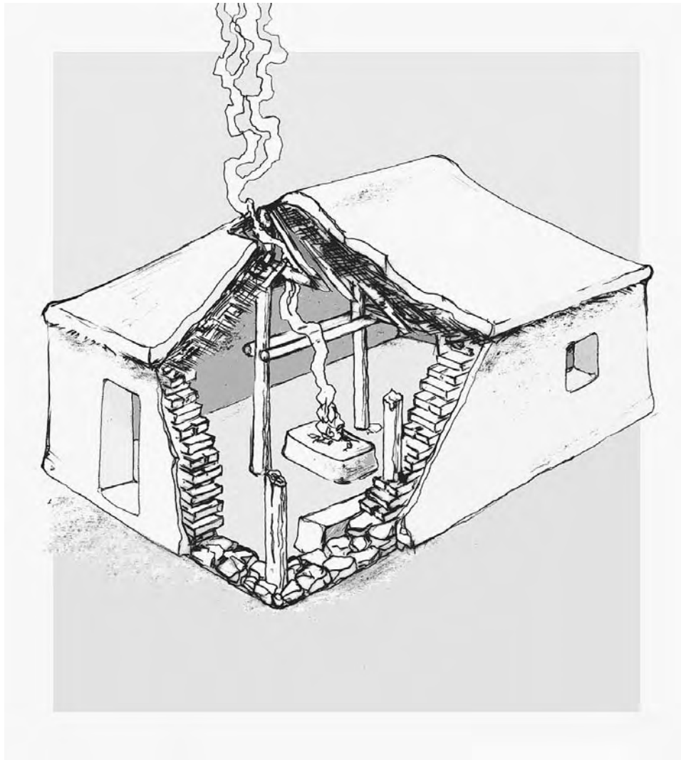
Fig. 2. Typical Neolithic house construction of stone foundations, mud-brick walls, and clay-covered wooden roof. REPRINTED WITH PERMISSION OF CAMBRIDGE UNIVERSITY PRESS AND GERARD MONTHEL.
