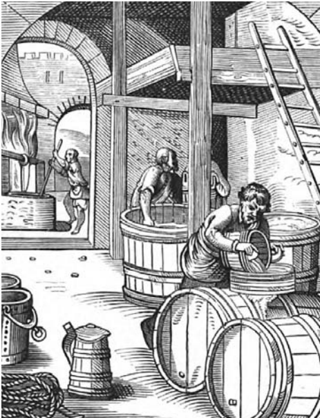
In a large, late medieval brewery, ale went through several stages of boiling, fermenting, and straining. Large oak barrels stored the finished product. (Paul Lacroix, Moeurs, Usage et Costumes au Moyen Age et a l'Epoque de la Renaissance , 1878)
