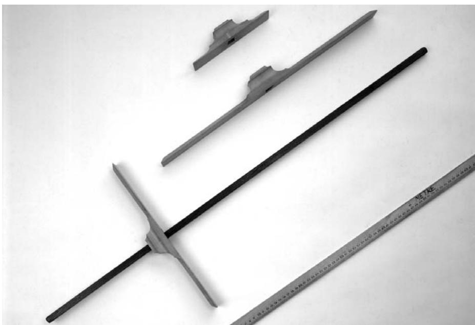
A modern yardstick sits next to a medieval cross-staff with two spare transoms that are longer and shorter than the one in use. The transom slid along the staff until its top and bottom were aligned with the horizon and a target star. Markings along the staff measured how far the transom had slid, and this could be translated into knowledge of where the ship was on a special map. (SSPL/Getty Images)
