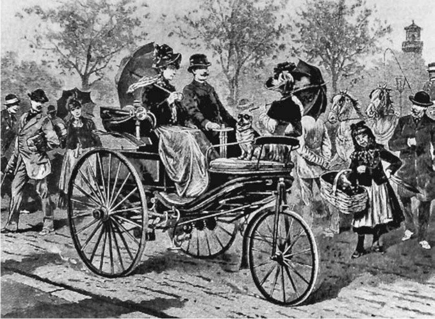
This print engraving, published in 1888 in the Leipziger Illustrierte Zeitung, is the first illustration of Karl Benz's Patent-Motorwagen, the world's first commercially available automobile using an internal combustion engine. Karl Benz completed the first model in 1885 and patented his new invention, based upon bicycle technology, the following year. (oldtimer-markt)
