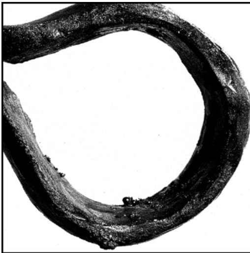
11.7 Brown globules of liquid at the internal face of an iron tool (Iron Age) excavated in the north of France. The alteration appeared after restoration (IRRAP).
