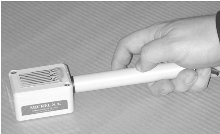
17.3 Taking readings from a prototype corrosion logger.
