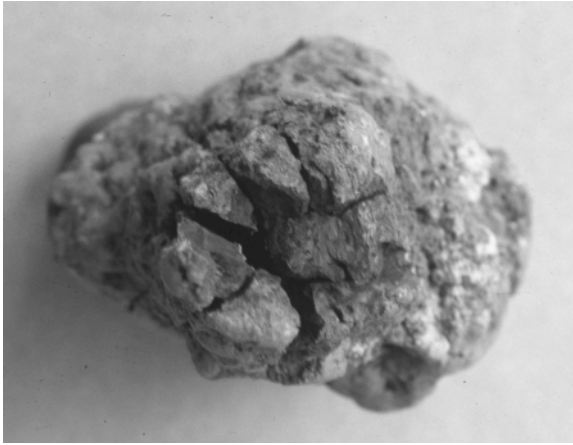
11.6 After excavation and before conservation treatment, breaking up of the extremity of a nail (Iron Age) due to corrosion (IRRAP).
