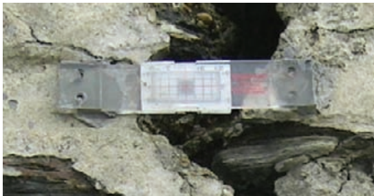
Figure 2.27 Graduated tell-tale bridging a fracture.
