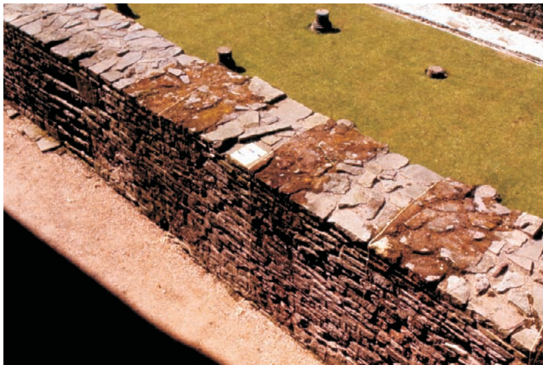
Figure 6.1 Biocide trials at Tintern Abbey in 1972, carried out by the Ancient Monuments Division and the Building Research Station. The objective was to compare different treatments against untreated controls, to identify the most effective and persistent materials to keep wall tops free of organic growth.
