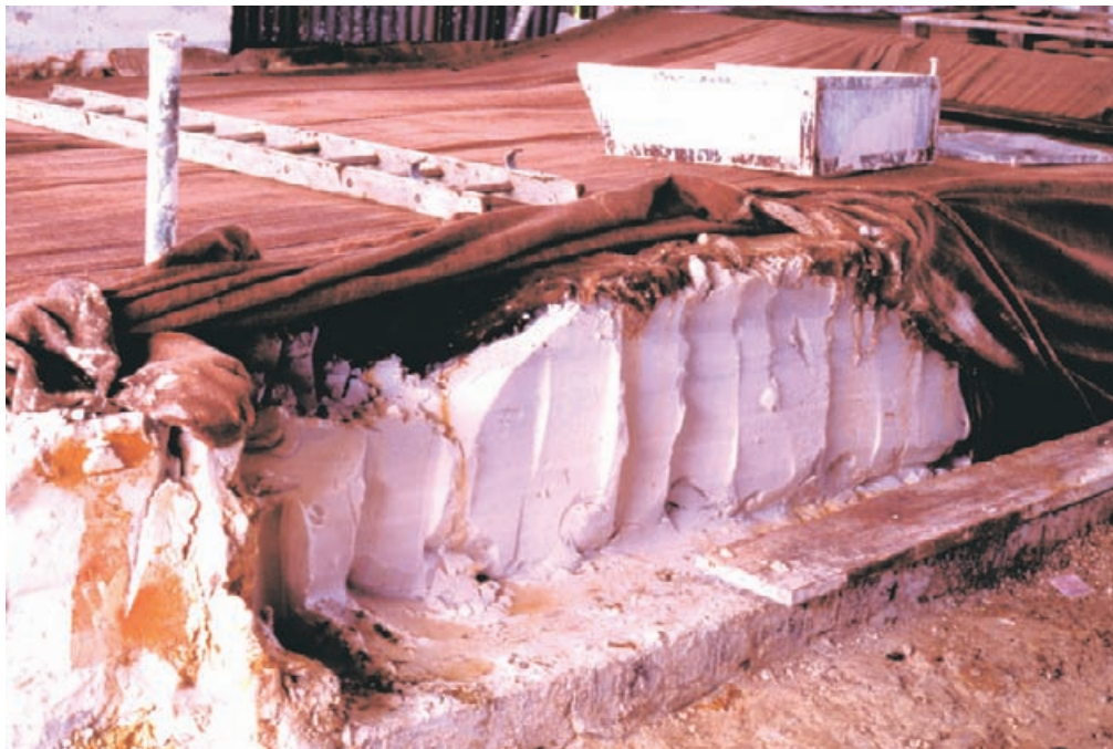
Figure 4.59 Mature lime putty which has been aged for three years exhibiting the right consistency for use as mortar. Bryn Gilby's lime production, South Wales.
