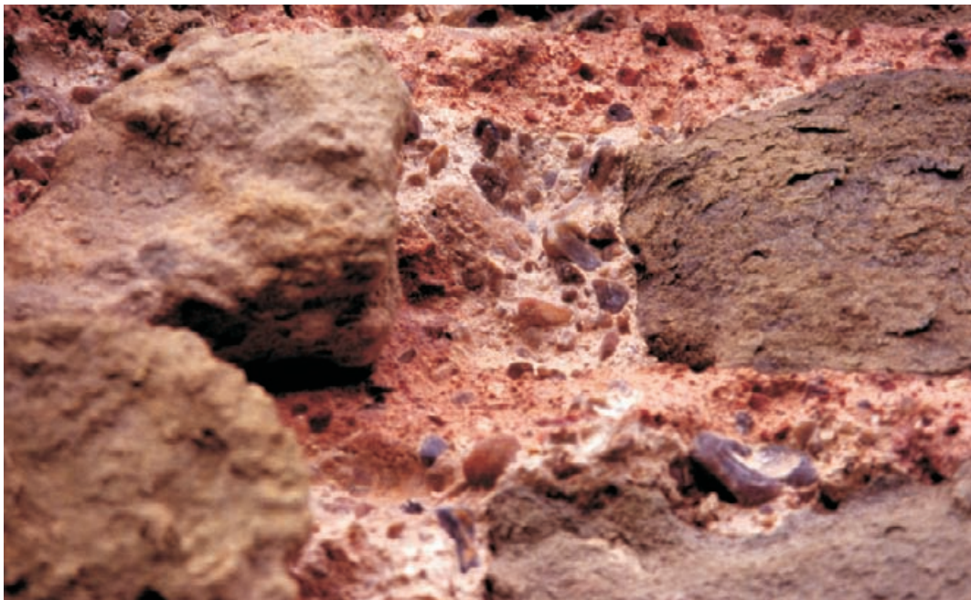
Figure 4.62 Roman mortar at Pevensey, Sussex, England showing the use of artificial pozzolan in the form of powdered brick or tile blended with large brick aggregate and lime. This mortar is extremely durable and has survived a marine environment for 2000 years.
