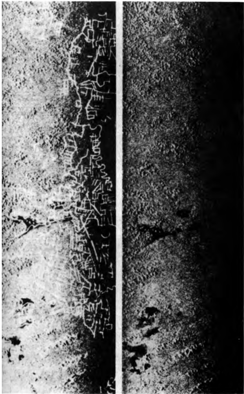
Comparison of radar imagery and regular aerial photograph taken over Guatemalan jungle. The lines in the radar imagery photograph prove to be irrigation canals dug by the ancient Maya. NASA
