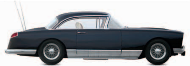
△ Facel Vega FVS 1954 Origin France Engine 5,801 cc, V8 Top speed 134 mph (216 km/h) One of the first European marques to use U.S. V8 power (in this case, from Chrysler), Facel Vega offered an outstanding "Grand Routier" in the extremely stylish FVS.
