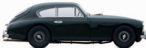
△ Aston Martin DB2/4 1953 Origin UK Engine 2,580 cc, straight-six Top speed 116 mph (187 km/h) Expensive and exclusive, with W.O. Bentley's twin-overhead-camshaft engine in a tubular chassis, the Aston Martin epitomized racing pedigree and class.
