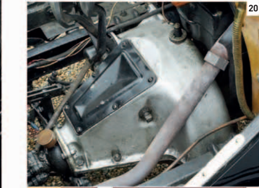
19. Trembler coils for ignition housed in box on dashboard 20. Transmission housing under the floor 21. Hood clip 22. Hood handle 23. Four-cylinder engine has a capacity of nearly 3 liters
