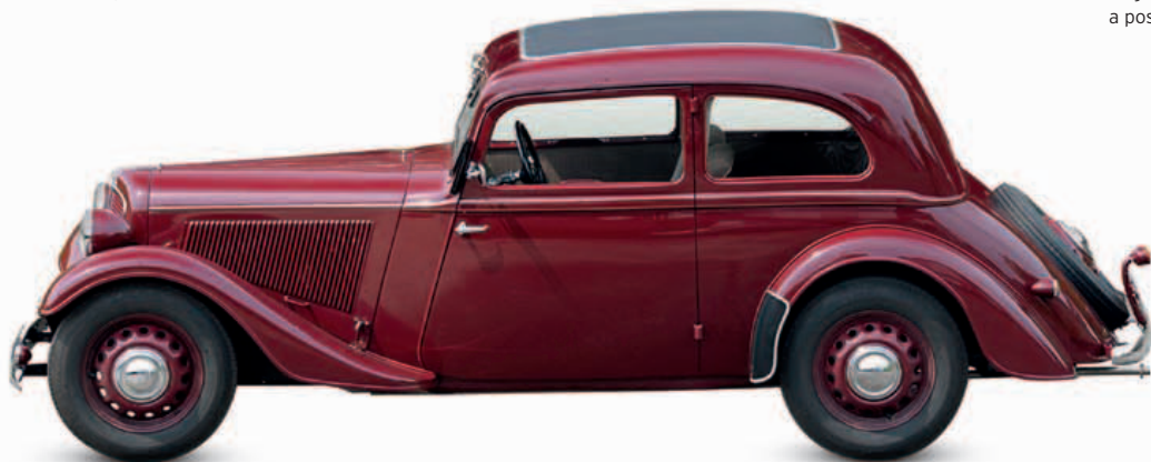
△ Adler Trumpf Junior 1934 Origin Germany Engine 995 cc, straight-four Top speed 57 mph (92 km/h)
