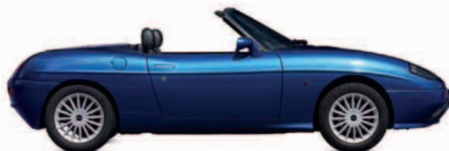
◁ Fiat Barchetta 1995 Fiat built the Barchetta on the Punto platform but, with a brand new twin-cam engine and beautiful, in-house-designed body, it's a far better sports car than many expect. Origin Italy Engine 1,747 cc, straight-four Top speed 118 mph (190 km/h)
