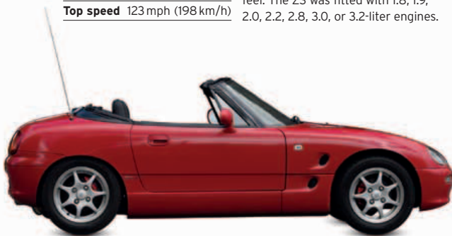
△ Suzuki Cappuccino 1991 Origin Japan Engine 657 cc, straight-three Top speed 85 mph (137 km/h)
