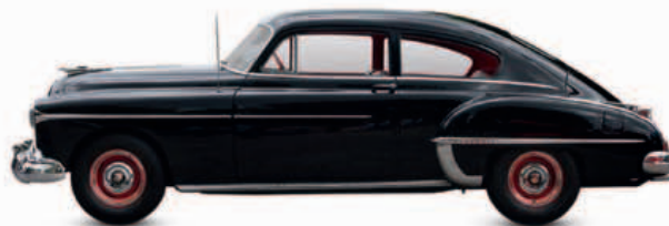
△ Oldsmobile 88 Club Sedan 1949 Origin USA Engine 4,977 cc, V8 Top speed 100 mph (161 km/h)
