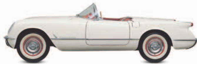
△ Chevrolet Corvette 1953 A Motorama dream car that made it to production, this was the first plastic-bodied car and represented a well-judged leap of faith by Chevrolet. Origin USA Engine 3,859 cc, straight-six Top speed 107 mph (172 km/h)
