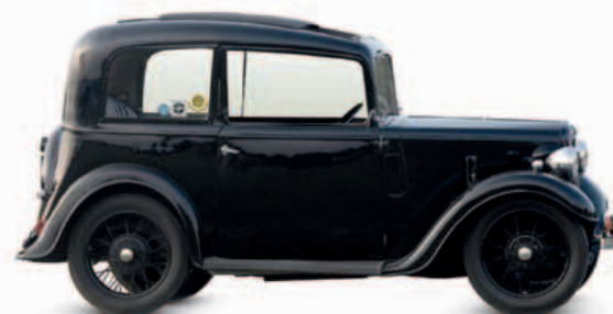
△ Austin Seven Ruby 1934 Origin UK Engine 747 cc, straight-four Top speed 50 mph (80 km/h)
