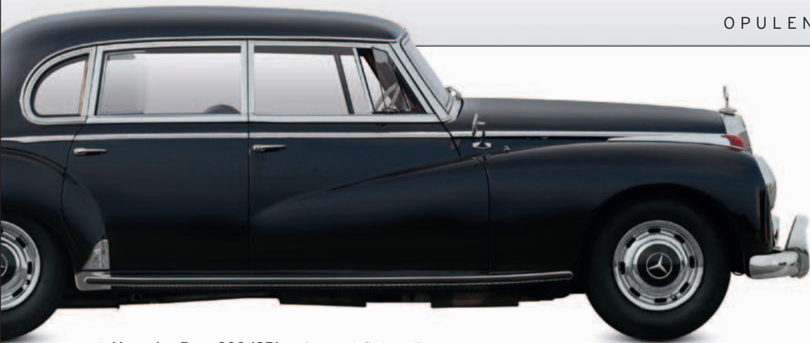
△ Mercedes-Benz 300 1951 Origin Germany Engine 2,996 cc, straight-six Top speed 103 mph (166 km/h) Germany's first prestige car after World War II was built with quality and durability as priorities. Around 1,000 a year were built over 10 years.
