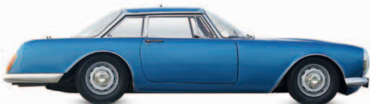
△ Facel Vega Facel II 1962 Origin France Engine 6,286 cc, V8 Top speed 133 mph (214 km/h)
