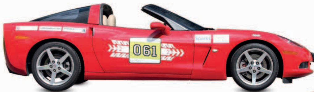
△ Chevrolet Corvette C6 2005 Origin USA Engine 5,967 cc, V8 Top speed 198 mph (319 km/h) Originally known as a car that had looks and power but little else, this Corvette can also boast of handling to match.
