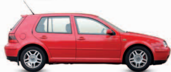
△ Volkswagen Golf GTI Mk4 1997 Origin Germany Engine 1,781 cc, straight-four Top speed 138 mph (222 km/h) The perennial hot hatch continued to sell well in its fourth generation with a turbo option. Volkswagen added a 3.2-liter 4x4 model too.
