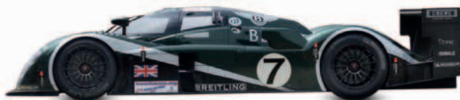
△ Bentley Speed 8 2001 Returning to Le Mans 73 years after its glory days in the 1920s, it took Bentley three attempts before winning once again in 2003. Origin UK Engine 4,000 cc, V8 Top speed 205 mph (330 km/h)
