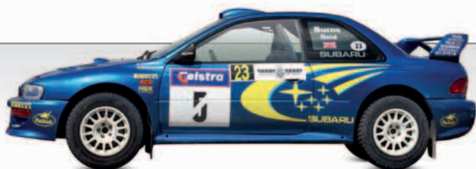
△ Subaru Impreza WRC 1999 Origin Japan Engine 1,994 cc, flat-four Top speed 140 mph (225 km/h)
