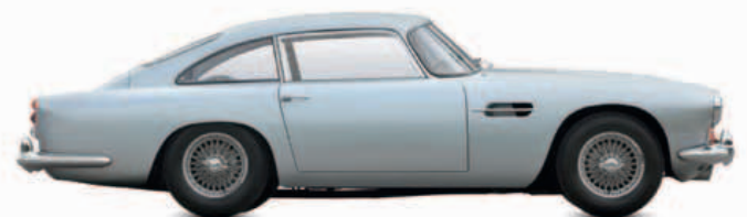
△ Aston Martin DB4 1958 Origin UK Engine 3,670 cc, straight-six Top speed 141 mph (227 km/h) By the end of the decade, the Aston Martin had grown into a true luxury supercar, with exotic Italian styling by Touring and 240 bhp from its new twin-cam engine.
