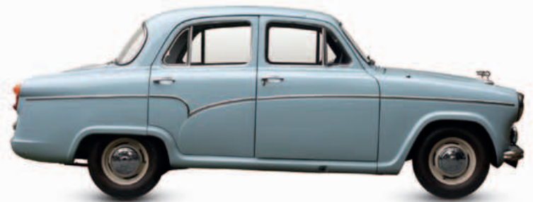
△ Austin A50/A55 Cambridge 1955 Origin UK Engine 1,489 cc, straight-four Top speed 75 mph (121 km/h)
