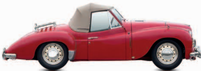
△ Jowett Jupiter 1950 Innovative but heavy, Jupiters enjoyed good handling thanks to a low, horizontally opposed engine. Jowett was too small to make it in quantity: 899 of these were sold. Origin UK Engine 1,486 cc, flat-four Top speed 84 mph (135 km/h)
