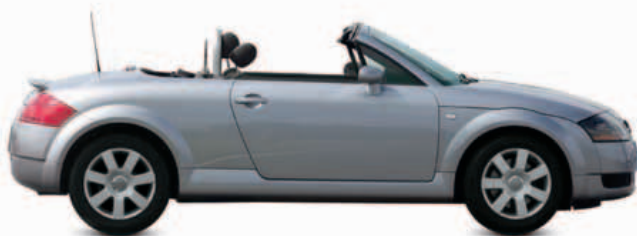
△ Audi TT Roadster 1999 Built in Hungary with either 4X2 or 4X4, Audi's TT uses Volkswagen Golf technology. It suffered bad press due to high speed instability, prompting recall modifications. Origin Germany Engine 1,781 cc, straight-four Top speed 138 mph (222 km/h)
