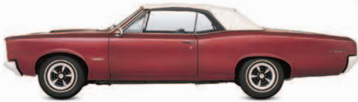
△ Pontiac Tempest GTO 1966 Origin USA Engine 6,375 cc, V8 Top speed 122 mph (196 km/h)
