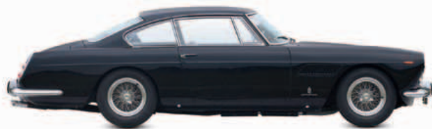
△ Ferrari 250GT 1956 Origin Italy Engine 2,953 cc, V12 Top speed 145 mph (233 km/h) Ferrari's first volume-production GT, the 250 boasted tremendous performance from the triple-Weber carburetor V12, within a luxurious 2+2 coupé styled by Pinin Farina.
