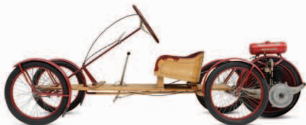
△ Briggs & Stratton Flyer 1919 Lawnmower engine maker Briggs & Stratton sold the Flyer until 1925. At $125, it was the cheapest new car ever. Origin USA Engine 201cc, one-cylinder Top speed 25 mph (40 km/h)
