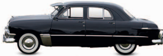
◁ Ford Custom V8 1949 Origin USA Engine 3,917 cc, V8 Top speed 85 mph (137 km/h)
