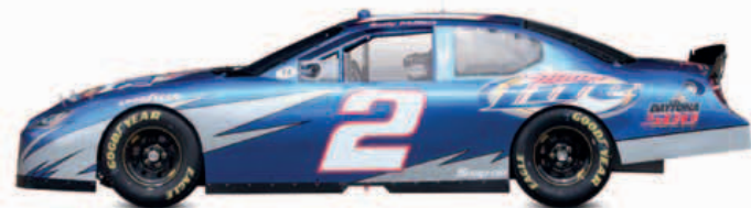
△ Dodge Charger 2005 Although branded a Charger, very little of the road car is used in NASCAR; just the engine within a purpose-built tubular chassis and sheet metal body. Origin USA Engine 5,860 cc, V8 Top speed 190 mph (306 km/h)
