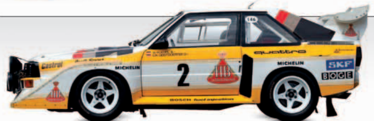
△ Audi Sport quattro S1 E2 1985 Origin Germany Engine 2,133 cc, straight-five Top speed 154 mph (248 km/h)
