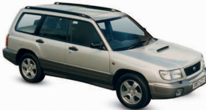
◁ Subaru Forester 1997 Origin Japan Engine 1,994 cc, flat-four Top speed 111 mph (179 km/h) Subaru's tough 4x4 station wagon offered comfortable road driving thanks to its low, flat engine. This made it more versatile than its competitors, though its looks were fairly uninspiring.
