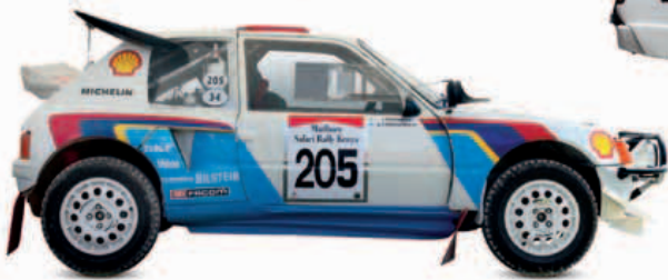
△ Peugeot 205 T16 Evo 2 1985 Origin France Engine 1,775 cc, straight-four Top speed 155 mph (249 km/h)
