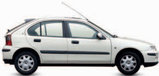
△ Rover 25 VVC 1999 Origin UK Engine 1,796 cc, straight-four Top speed 127 mph (204 km/h) Based on engineering from Honda pre-1994, the 25 was well equipped and good value, with engines from 1.1 to 2.0 liters.
