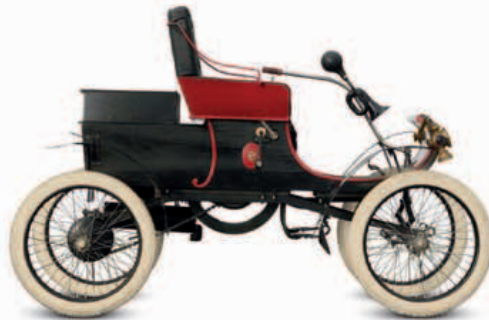
△ Oldsmobile Curved Dash 1901 Origin USA Engine 1,564 cc, single-cylinder Top speed 20 mph (32 km/h)
