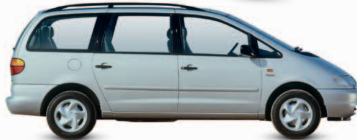
◁ Volkswagen Sharan 1995 Origin Germany/Portugal Engine 1,984 cc, straight-four Top speed 110 mph (177 km/h) Also sold as the SEAT Alhambra and produced alongside the similar Ford Galaxy, Volkswagen's people-carrier didn't have the best reliability record. Engines ranged from 1.8 to 2.8 liters.
