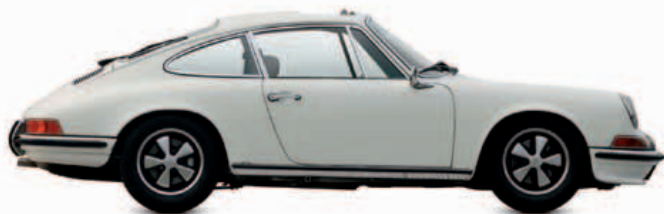
△ Porsche 911S 2.2 1970 The 911 gained improved handling for the 1970s by moving the rear wheels back by 2.2 in (5.5 cm) and the fuel-injected S took full advantage, becoming a junior supercar.
