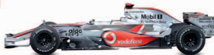
△ McLaren-Mercedes MP4/23 2008 In only his second season of Formula 1 Grand Prix racing, Lewis Hamilton became the youngest world champion ever at the wheel of this car. Origin UK Engine 2,400 cc, V8 Top speed 200 mph (322 km/h)
