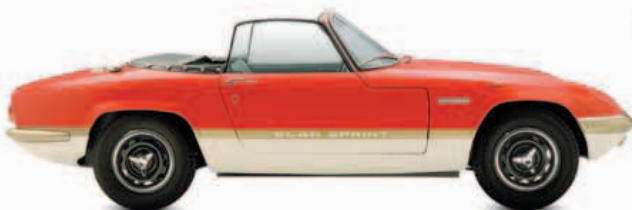
△ Lotus Elan Sprint 1971 Origin UK Engine 1,558 cc, straight-four Top speed 120 mph (193 km/h)
