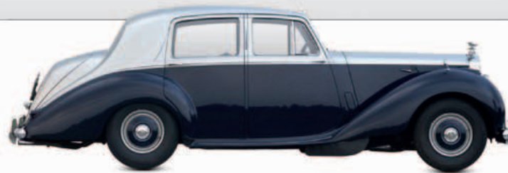
△ Rolls-Royce Silver Dawn 1949 Origin UK Engine 4,566 cc, straight-six Top speed 87 mph (140 km/h)
