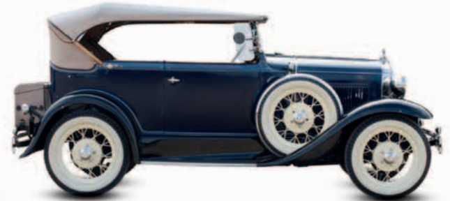
△ Ford Model A 1927 The Model A was a mass-production car for middle America, but it still managed to exude gangster-movie style. It was given strong body colors and whitewall tires. Origin USA Engine 3,285 cc, straight-four Top speed 60 mph (97 km/h)
