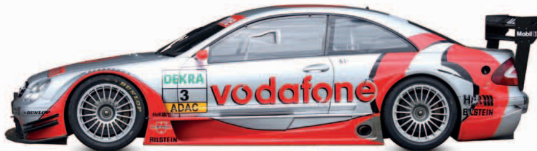
△ Mercedes-Benz CLK DTM 2003 Based on a tubular-steel chassis and powered by V8 engines, German Touring Cars have only a passing resemblance to the production models they represent. Origin Germany Engine 4,000 cc, V8 Top speed 180 mph (290 km/h)
