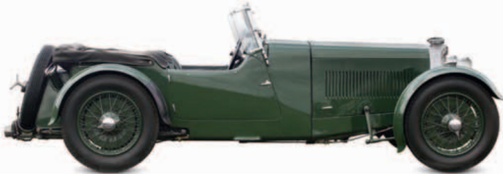
▷ Alfa Romeo 8C 2600 1933 Origin Italy Engine 2,556 cc, straight-eight Top speed 105 mph (169 km/h)
