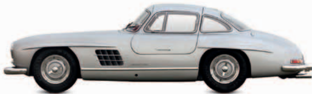
△ Mercedes-Benz 300SL 1954 Origin Germany Engine 2,996 cc, straight-six Top speed 129 mph (208 km/h) One of the most iconic cars of the 1950s, the 300SL with its gull-wing doors and 250 bhp fuel-injected, dry-sump engine was an outstanding sports coupé.
