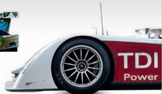
△ Audi R8 2000 One of the most successful endurance racing cars ever, the R8 won Le Mans five times over six years, only losing out to Audi-owned Bentley in 2003. Origin Germany Engine 3,600 cc, V8 Top speed 211 mph (339 km/h)
