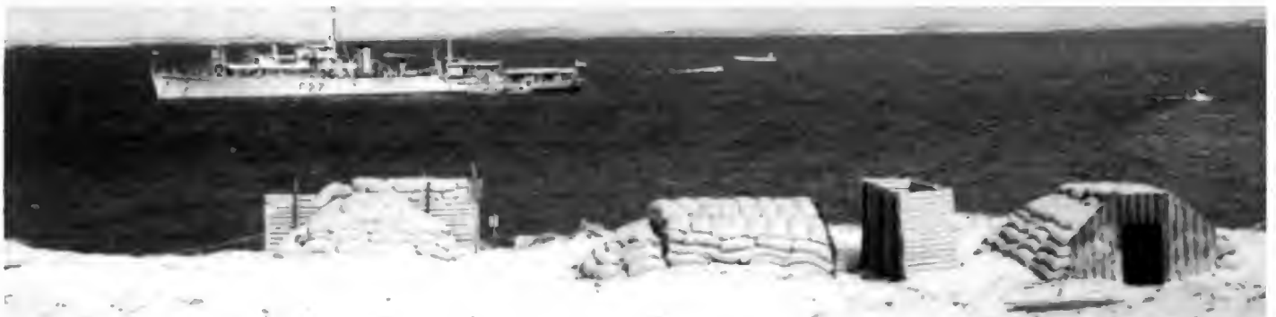
Fig. 12.1, Andersons at 1380 ft range from bomb ship shown in the photo, moored 400 yards off shore.
