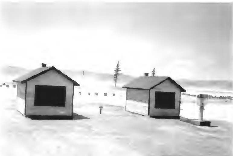
ENCORE test, Nevada, 1953 10' x 12' wooden houses with 4' x 6' windows 17 calories/sq. cm thermal flash
