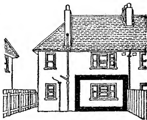
In a house with only two floors and without a cellar, choose a room on the ground floor so that you have protection overhead
