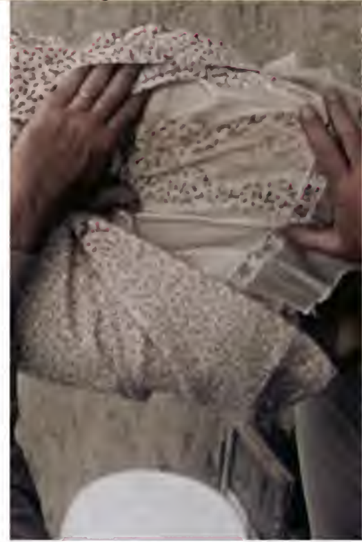
Above and below: clothing fails to ignite on mannequins located at 7000 feet from ground zero, 29 kt Teapot-Apple 2, 5 May 1955.
