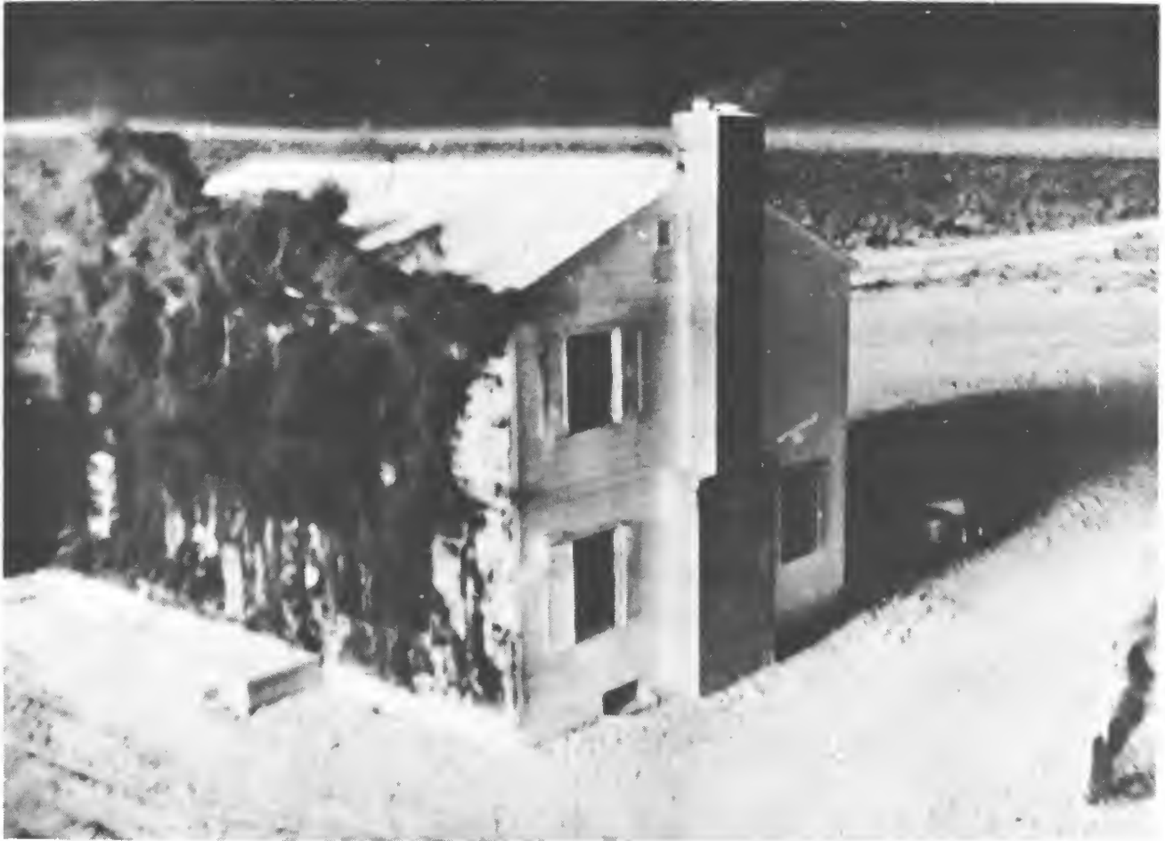
Figure 7.33a. Thermal effects on wood-frame house 1 second after explosion (about 25 cal/sq cm).
