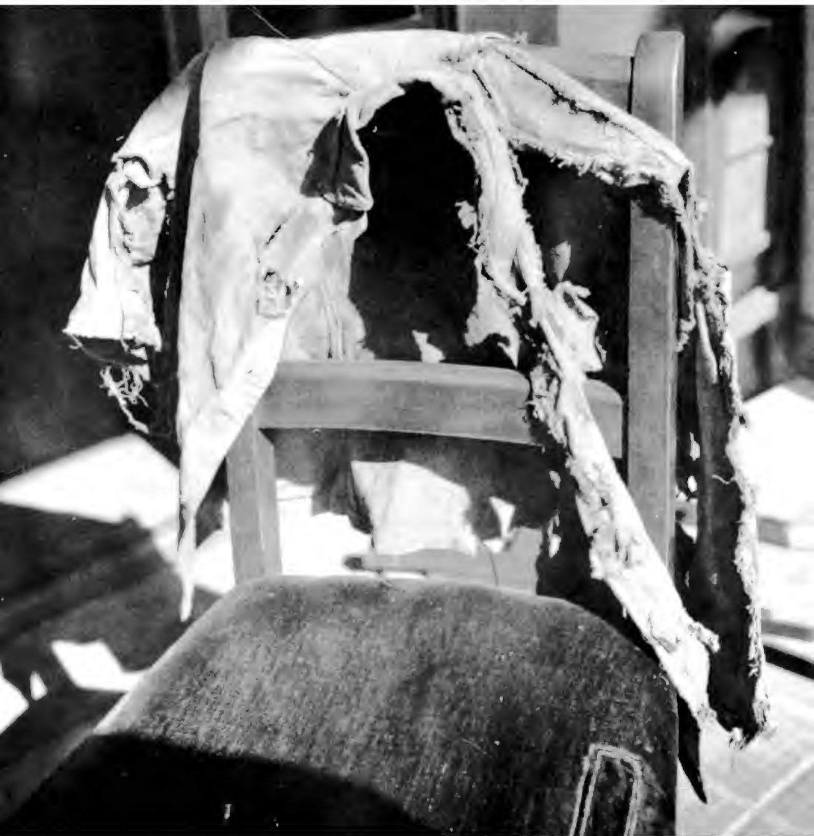
PHOTO 38 IX. Shows partly burned coat of boy who was in open near City Hall (Building 28) 3,800 feet from AZ.
