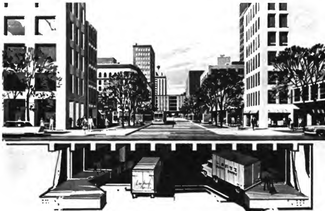
Proposed Dual-Use Shelters for Manhattan. (Interconnecting Traffic Tubes and Underground Parking Areas)
