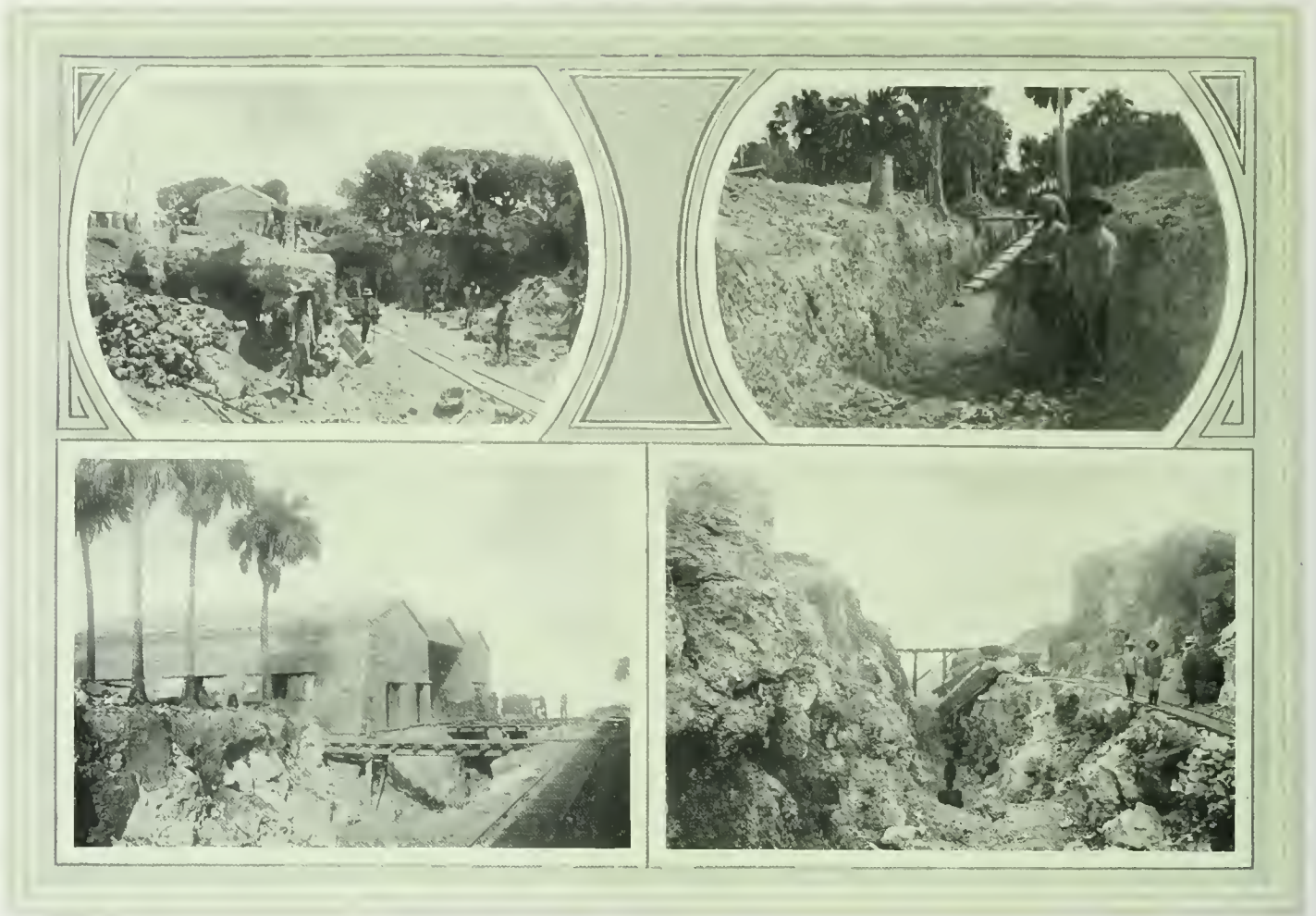
RASA ISLAND PHOSPHATE CO., LTD.: TRUCKING THE ROCK AWAY—TRENCHING FOR PHOSPHATIC ROCK—THE STORING AND DESPATCHING SHEDS—THE BIG QUARRY NEAR THE WATERFRONT
