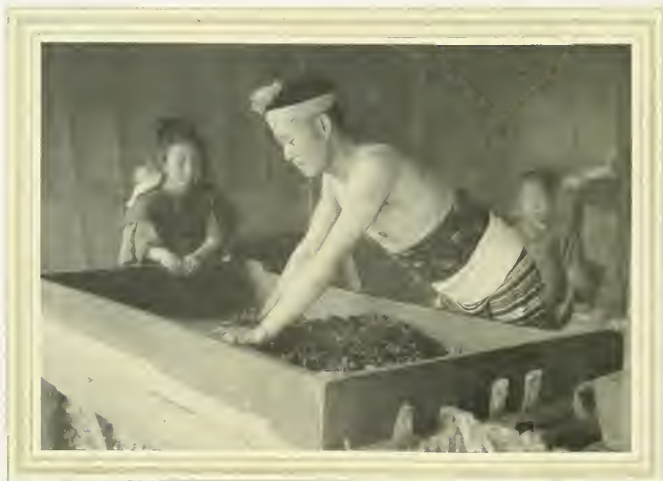
DRYING THE TEA OVER A CHARCOAL FIRE, AS IT IS DONE IN A SMALL FACTORY
