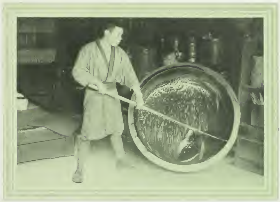
THE PROCESS OF CONDENSING LIQUID LACQUER IN THE SUN
