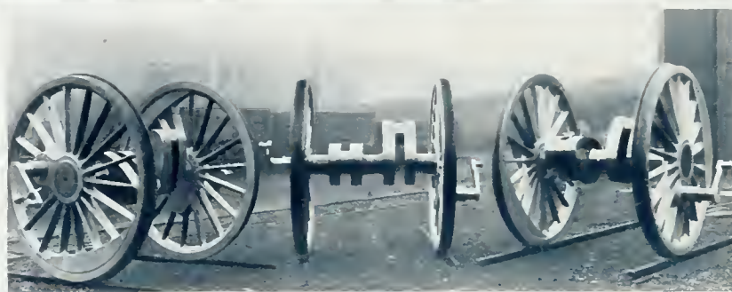
THOS. FIRTH & SONS, LTD.: STAMPS AND OTHER MINING BATTERY PARTS AND LOCOMOTIVE DRIVING WHEELS MANUFACTURED BY THE FIRM
