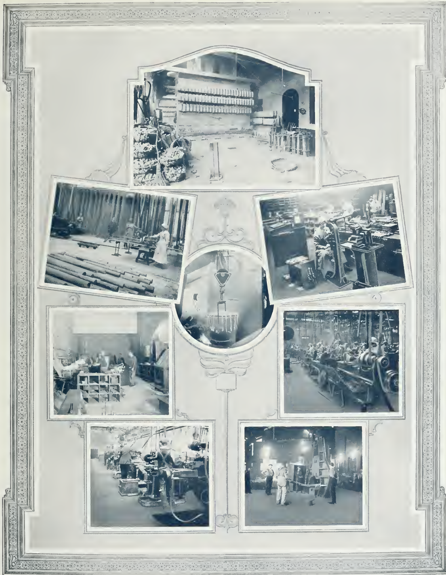
ARTHUR BALFOUR CO., LTD.: INTERIOR OF CRUCIBLE STEEL MELTING DEPARTMENT—SAWING A STEEL BAR TO LENGTH FOR TWIST DRILLS—(CENTRE) ELECTRIC FURNACE—INSPECTION DEPARTMENT IN TWIST DRILL AND CUTTER WORKS—TWIST DRILL AND CUTTER HARDENING SHOP—THE TURNING OF TWIST DRILLS—A FEW OF THE MILLING MACHINES IN ONE OF THE BAYS ENGAGED IN PRODUCING MILL CUTTERS, ETC.—HAMMERING A BAR OF STEEL
