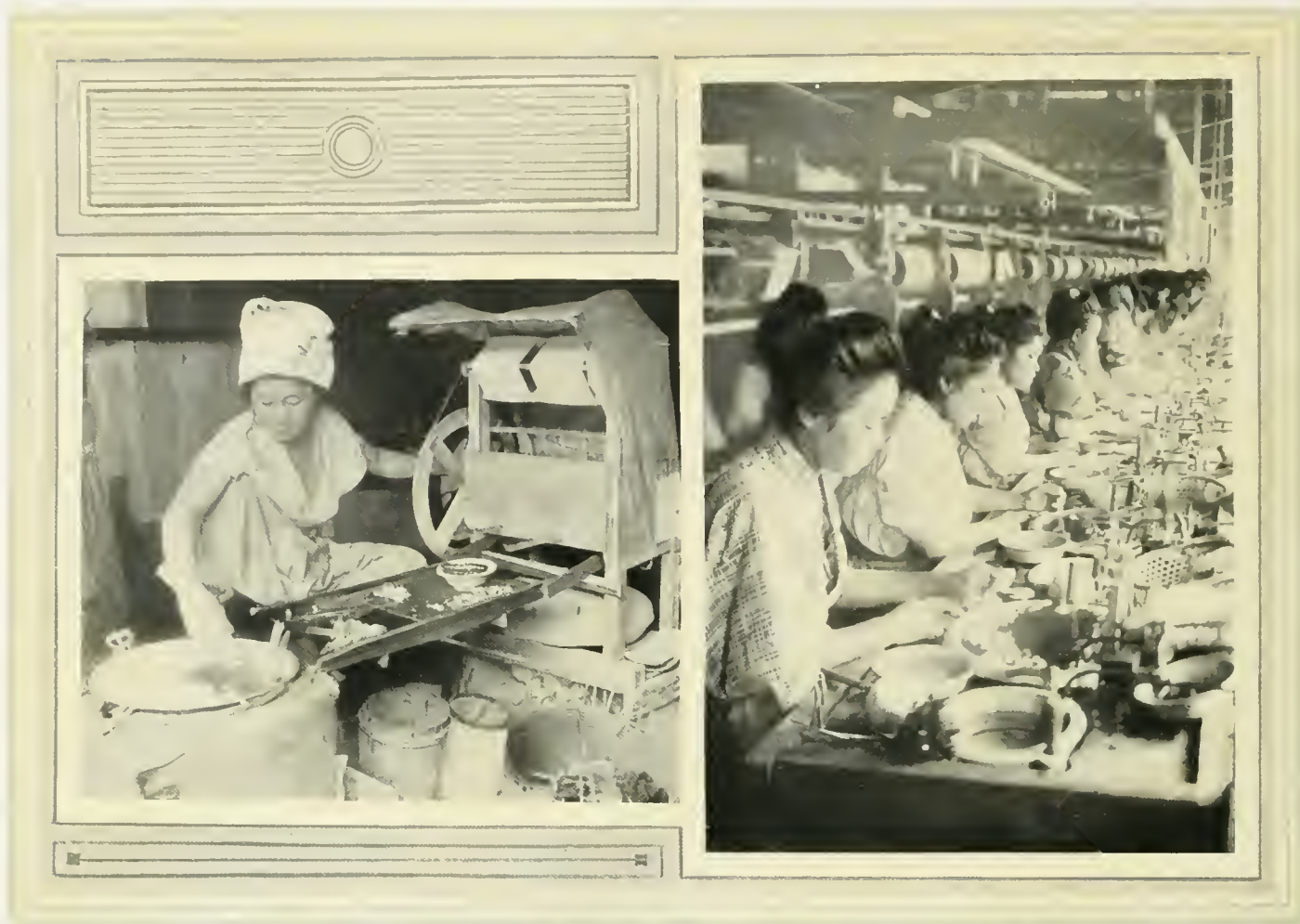
THE PROCESS OF IMMERSING THE COCOON IN BOILING WATER PRIOR TO UNWINDING THE SILK, AS CARRIED ON IN THE HOME AND IN THE FACTORY
