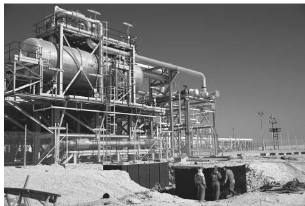
A degassing station in Dukhan, Qatar's center for oil production and the country's only onshore oil field. Dukhan, which was first drilled in 1939, contains three reservoirs which supply the majority of Qatar's oil. © CHRISTINE OSBORNE/CORBIS. REPRODUCED BY PERMISSION.
