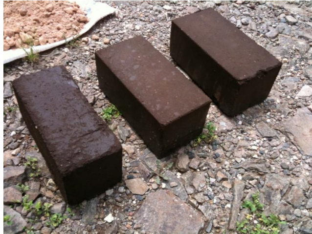
Picture 26. Water was poured on 3 blocks from group 1-3 (0 %, 4 % and 8 %-cement). The water had done much more damage to the 0% cement block than to the 4 % and 8% cement blocks. [5]
