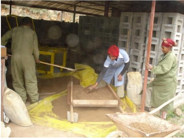
Picture 18 (left). The soil is being screened... [5]
