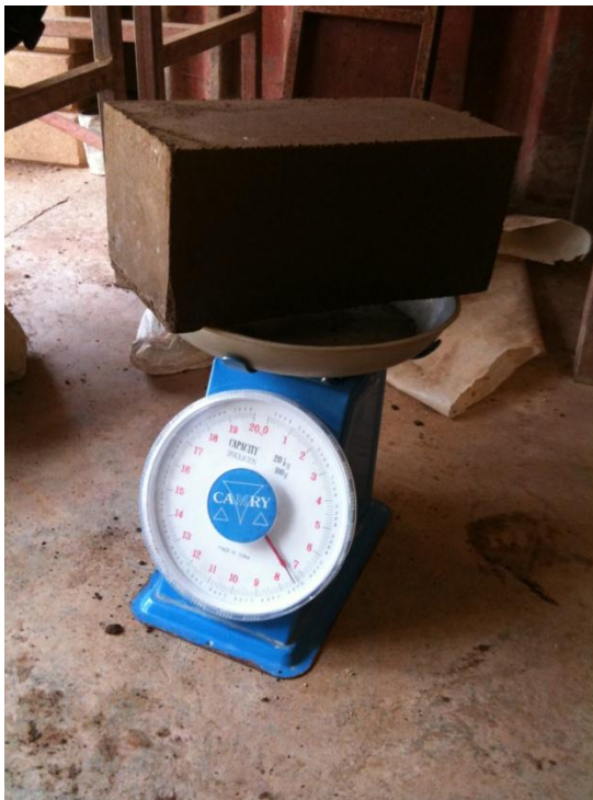
Picture 24 (left). The pressed blocks were weighed... [5]
