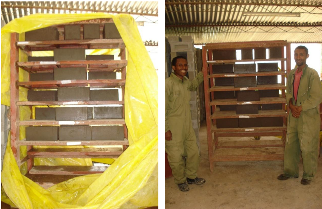
Picture 22 (left). The pressed blocks were stored on shelves, covered with a plastic sheet and sprinkled with water once per day during the wet-curing. [5]
