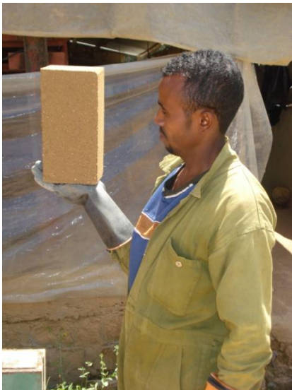
Picture 10 (Left). An employee at STVC holding a manually pressed CSSB. [5]
