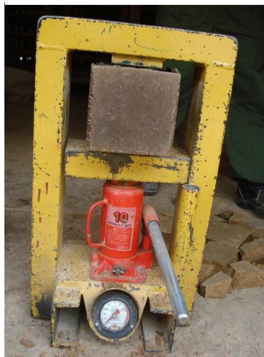
Picture 25 (right). ...before being placed between the stamps of the Compressive strength testing machine [5]
