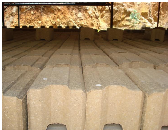
Picture 4. Interlocking CSSB at Selam Technical and Vocational Center, Addis Abeba. [5]
