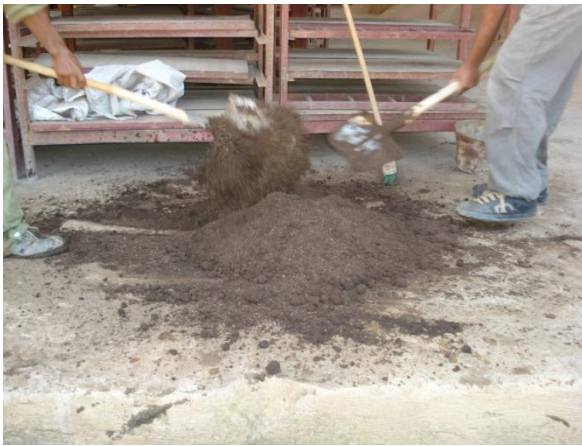
Picture 20 (left). Water was then added and the different components were wet-mixed. [5]
