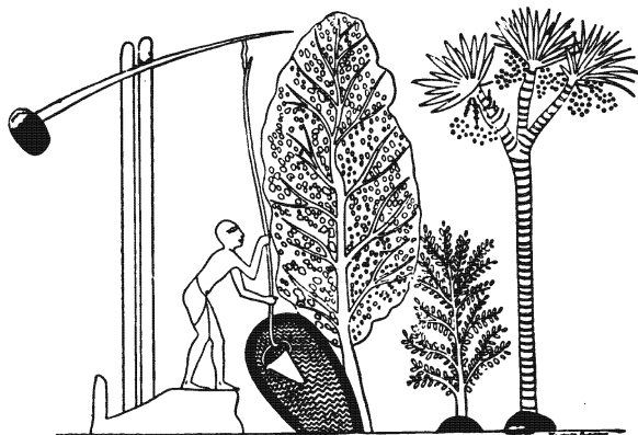
Fig. 59.—The Balance for drawing Water : the Shadouf .
